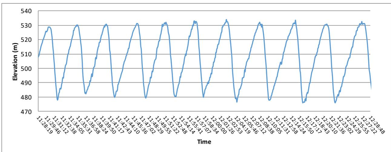
Figure 11: Skidder elevation changes of from one period on Day 1. Each sinus curve is one extraction cycle: the skidder descends to pick up the load (dip), then comes back up to take its load to the landing (peak).
