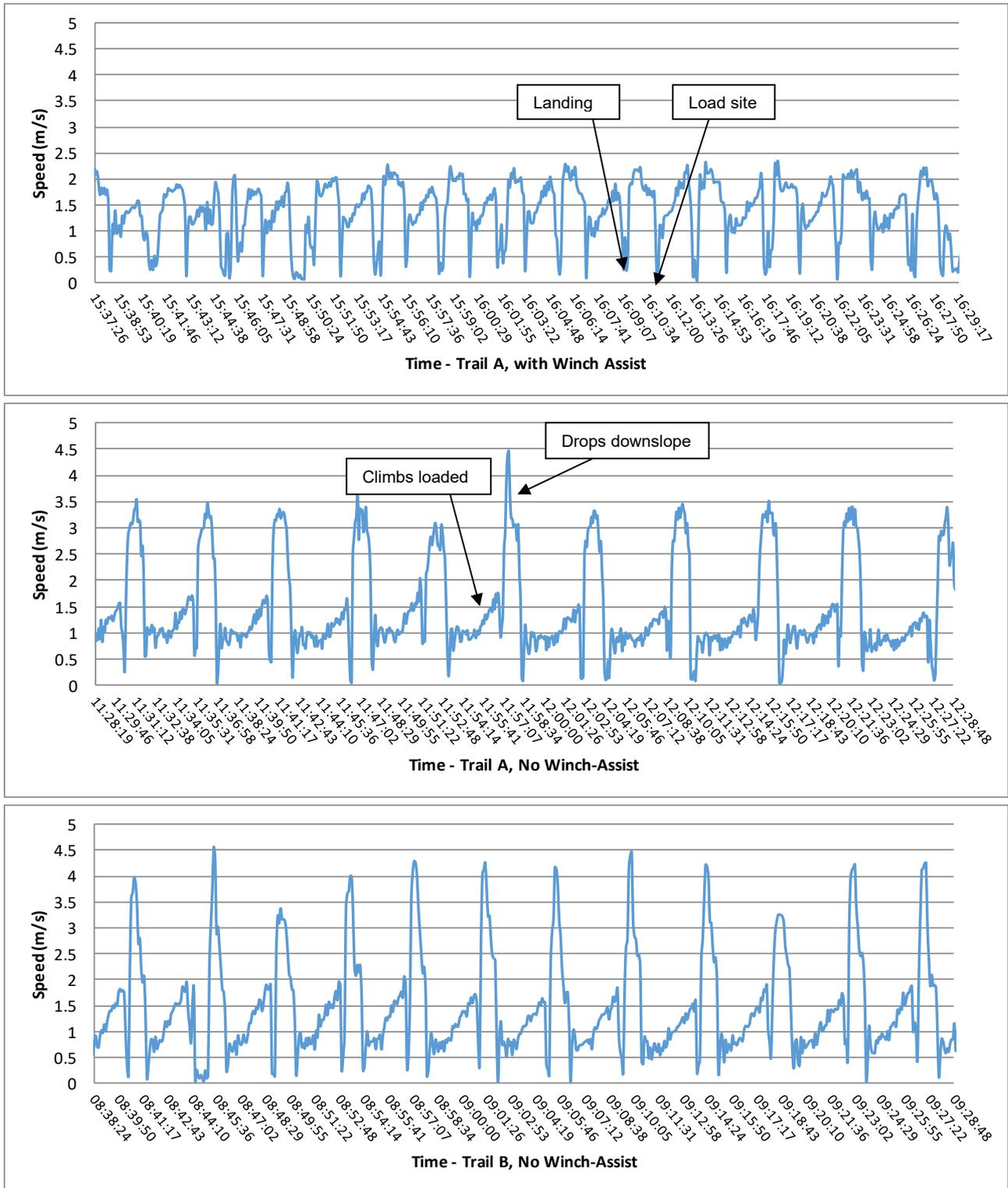
**Figure 12: Skidder speed charts. They show the high peak and fast speed ramp on the travel empty down the hill and the much smaller peak and slower speed ramp as the loaded skidder struggled uphill.**
