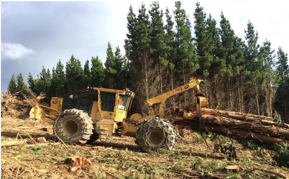
**Figure 1: Tigercat 632E skidder hauling logs to landing.**
