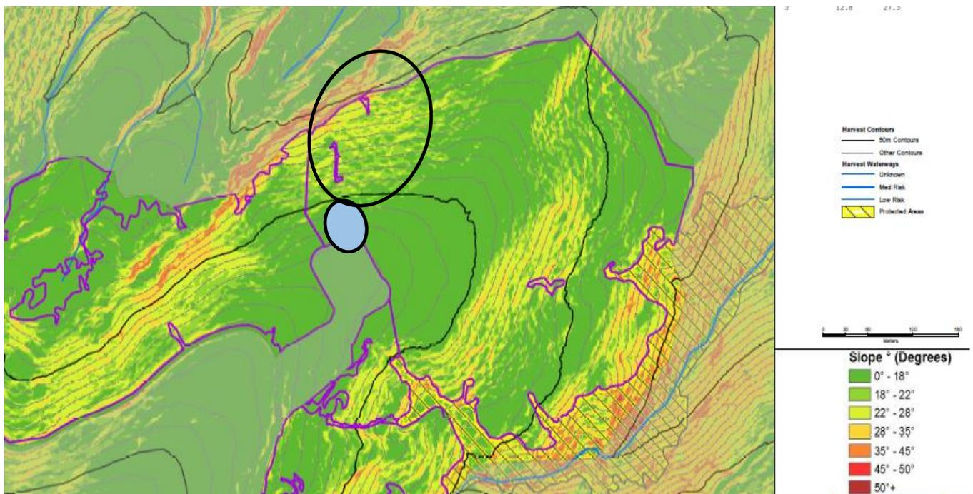
**Figure 2: Section of harvest area showing slope by category. The blue circle shows location of the landing, the area circled was the skidder study.**
