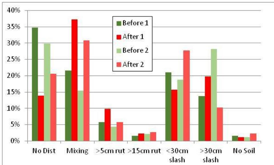
**Figure 15: Soil disturbance recorded over the two transects before and after skidding**
