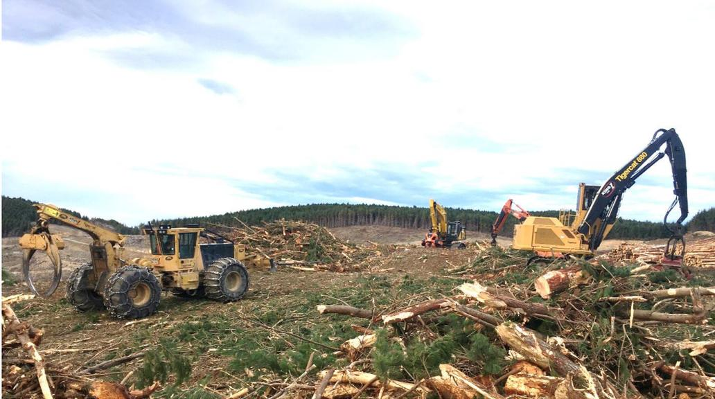
**Figure 4: Landing used during the initial study at Castle Downs Forest. The skidder was lined up with the TimberMax winch assist unit (centre). The stems were dropped to the left of the processor (shown on the right).**
