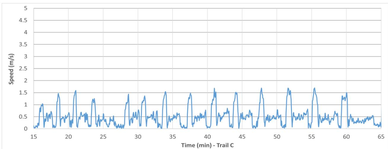
**Figure 13: Skidder speed chart for Blackmount (Path 3) where the skidder was winch-assisted by the TimberMax on the steeper slope.**
