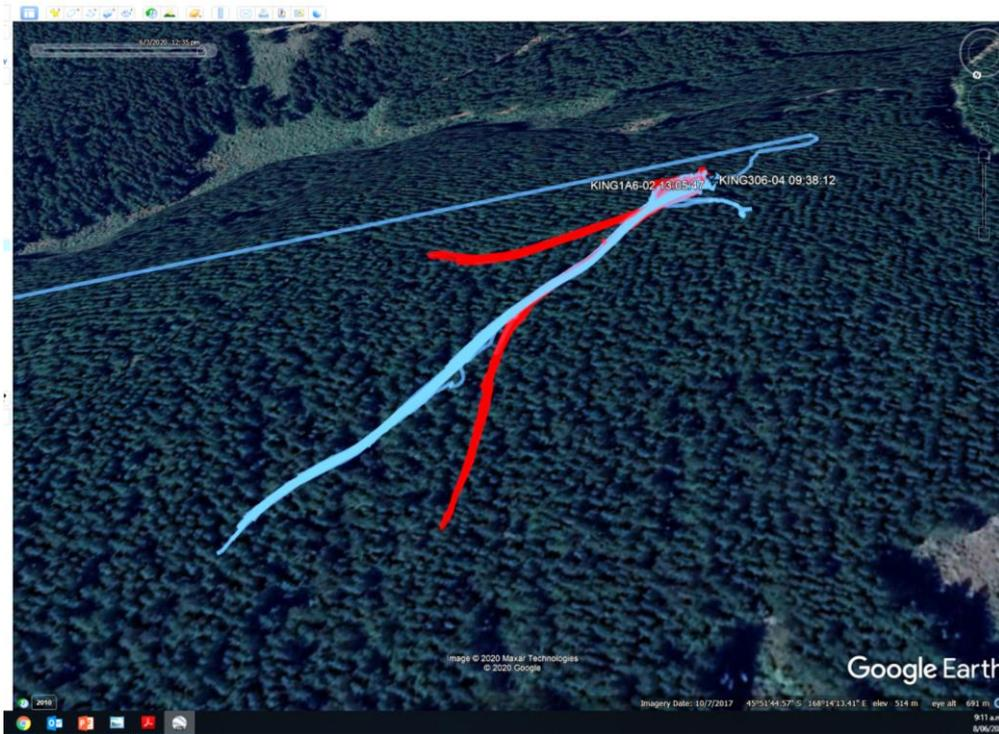
**Figure 8: Winch-assisted Tigercat 632E skidder navigating 21 degree (38%) slope, was fitted with a GPS unit to track its location, speed and change in altitude.**
