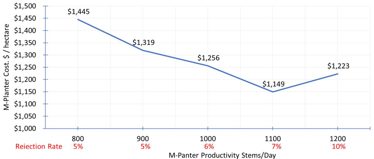
Figure 2. M-Planter Operational Costs and Rejection Rates Across Different Planting Productivity Levels
