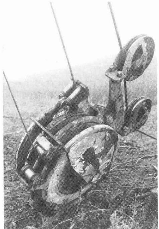
Figure 2 : The Interstate I-DLC 36 carriage used on the 171 Madill
