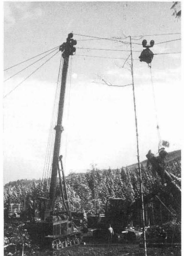
Figure 1: The new 171 Madill hauler, a machine with potential for logging new crop.
