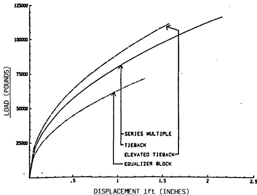
Figure 2 - Model load-deformation curves for four rigging configurations. The curves end at the load where system failure occurs
