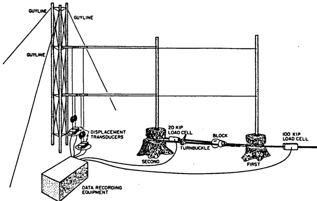
*Figure 3 - Side view of the data collection rigging configuration for the series multiple system*
