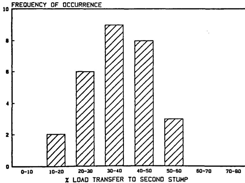
Figure 4 - Frequency of load transfer - skyline to second stump
