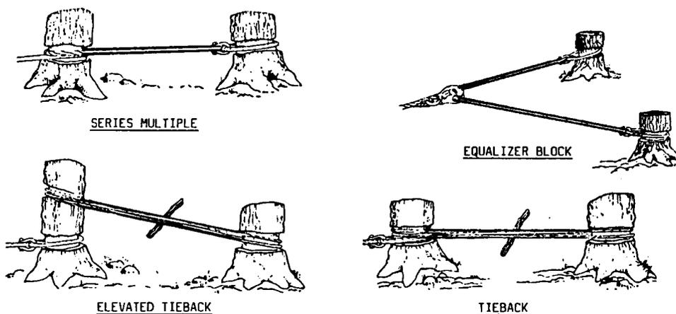
*Figure 1 - Multiple anchor rigging configuration*
