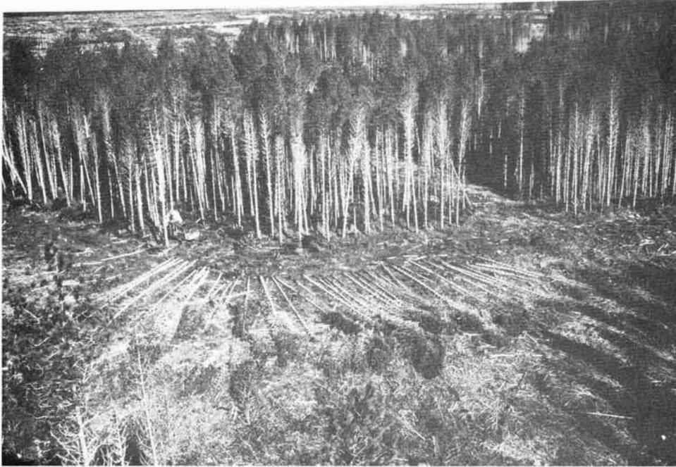
*Hitachi feller-buncher placing trees to assist delimiting*
