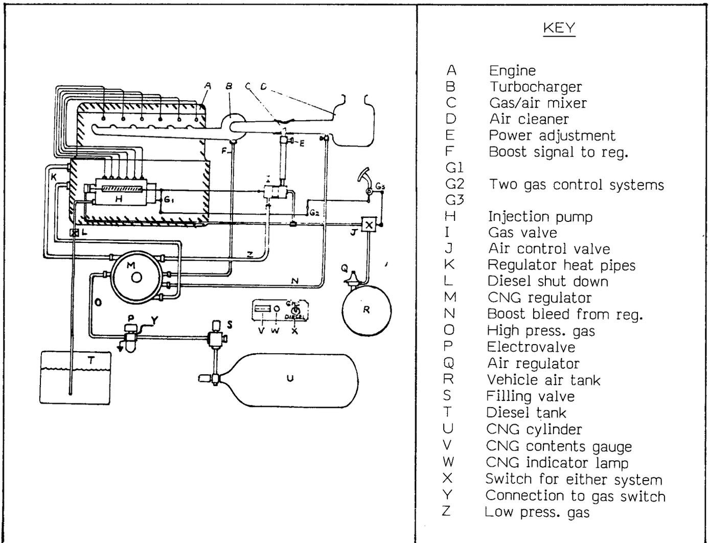
Fig. 1 - Layout of CNG-diesel system
