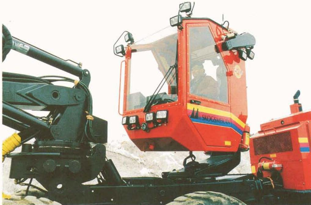
*Figure 1 - The self-levelling and swivelling cab suspended from an arched column attached to a swivelling socket*
