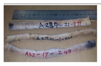
Peeling trials using 30-year-old E. globoidea were undertaken in collaboration with Nelson Pine Industries Ltd. The trials demonstrated that veneers of suitable quality could be obtained from the trees, and also demonstrated the importance of low growth strain to maximise veneer yields. Image below shows a high quality veneer sheet (top) and a sheet with severe splitting (bottom).
