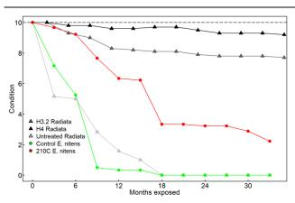
Figure: Fungus cellar stakelet results following 33 months of exposure. A condition of 10 indicates no sign of decay, and 0 indicates complete failure from decay.
