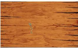
Glue bond trials were undertaken on young *E. bosistoana* and *E. quadrangulata* peeled at NPI. Results indicate that the standard phenolic resins used to bond radiata pine are likely to need to be modified to bond the *E. bosistoana* and *E. quadrangulata* veneer. Image below shows the veneer sheets that were supplied for the testing.
