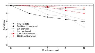
Figure: Fungus cellar stakelet results for modified C. lusitanica following 12 months exposure
