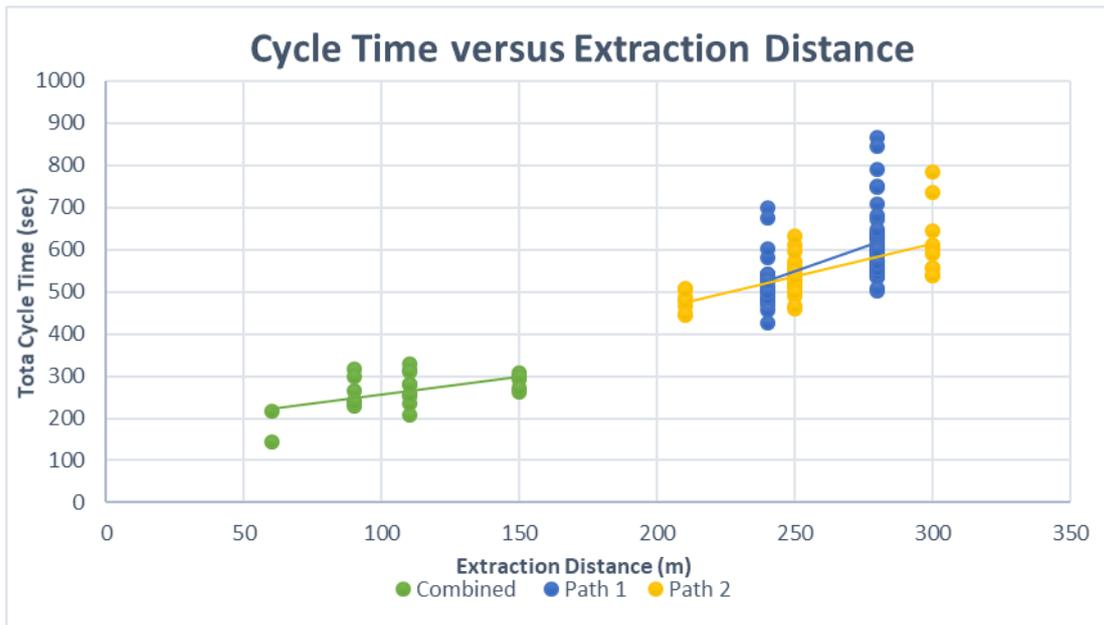
**Figure 11: Cycle times recorded at varying measured extraction distances**
