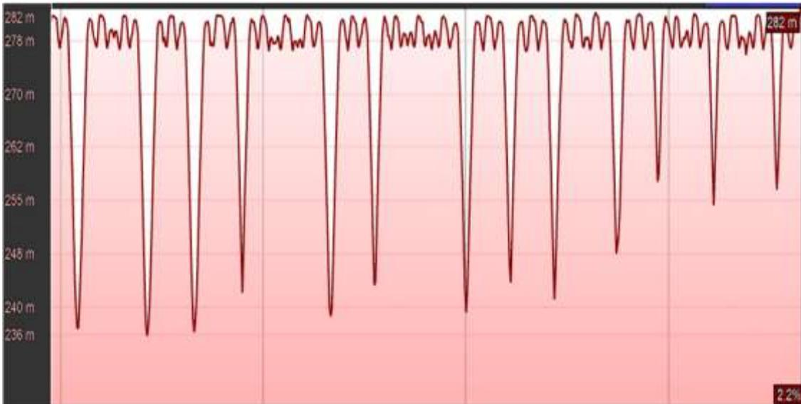
**Figure 14: Skidder elevation changes from one period on Day 2. Each drop in elevation is one extraction cycle with the skidder travelling downhill to pick up the load.**
