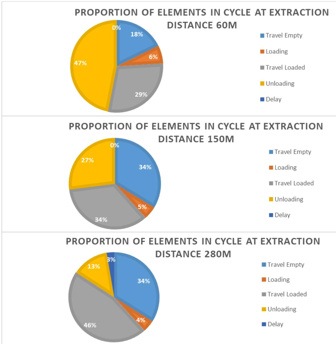
**Figure 10: Proportion of total cycle time for each element extraction distances of 60m, 150m and 280m.**
