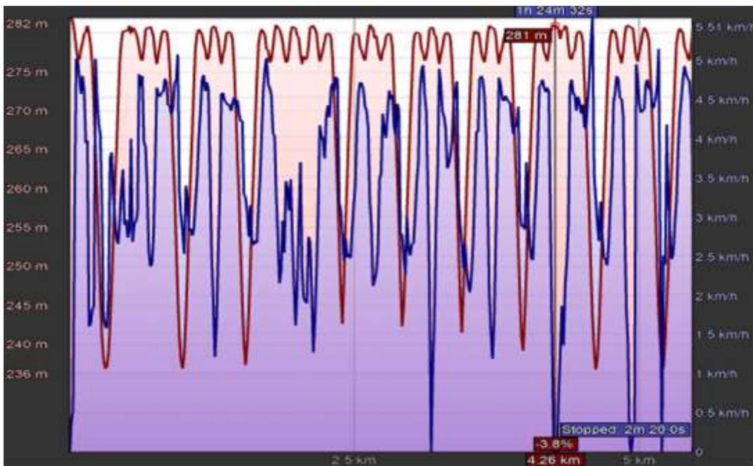
**Figure 15: Changes in elevation (red) and velocity of skidder (blue)**
