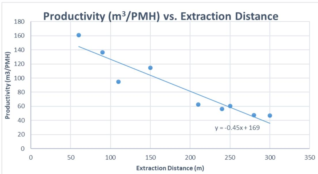
**Figure 12: Productivity of average cycle times at each extraction distance**
