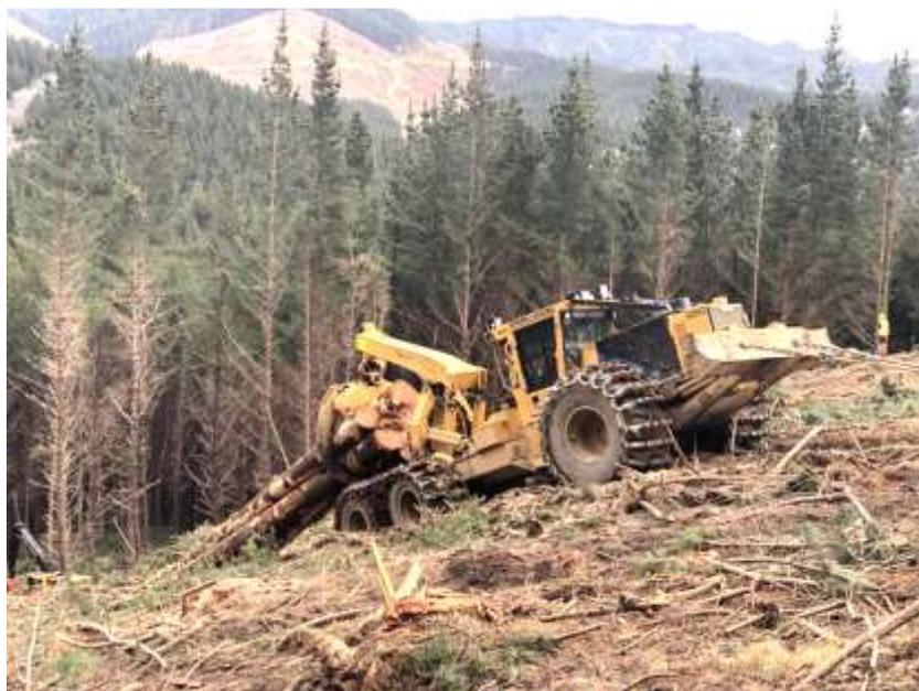
**Figure 1: Tigercat 635G skidder hauling logs to landing with traction assistance.**
