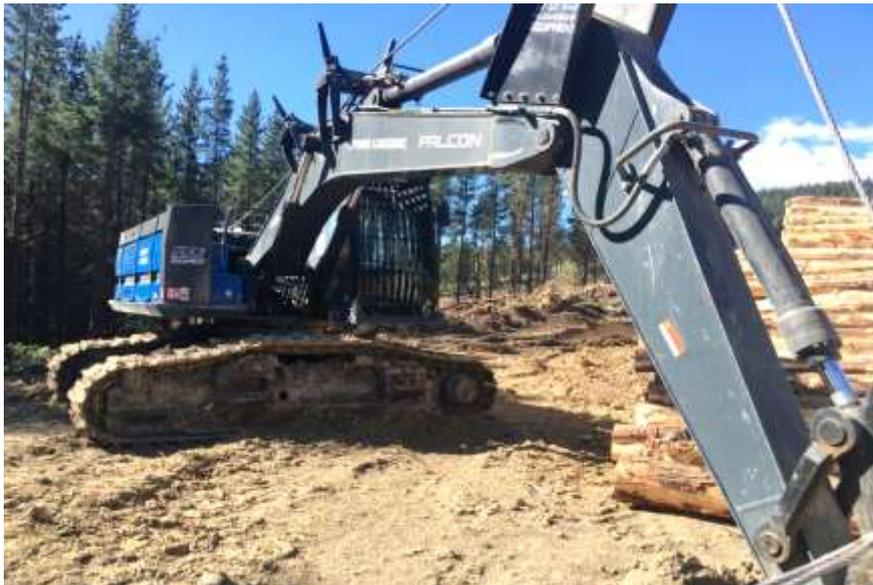
*Figure 6: Falcon Winch Assist machine*
