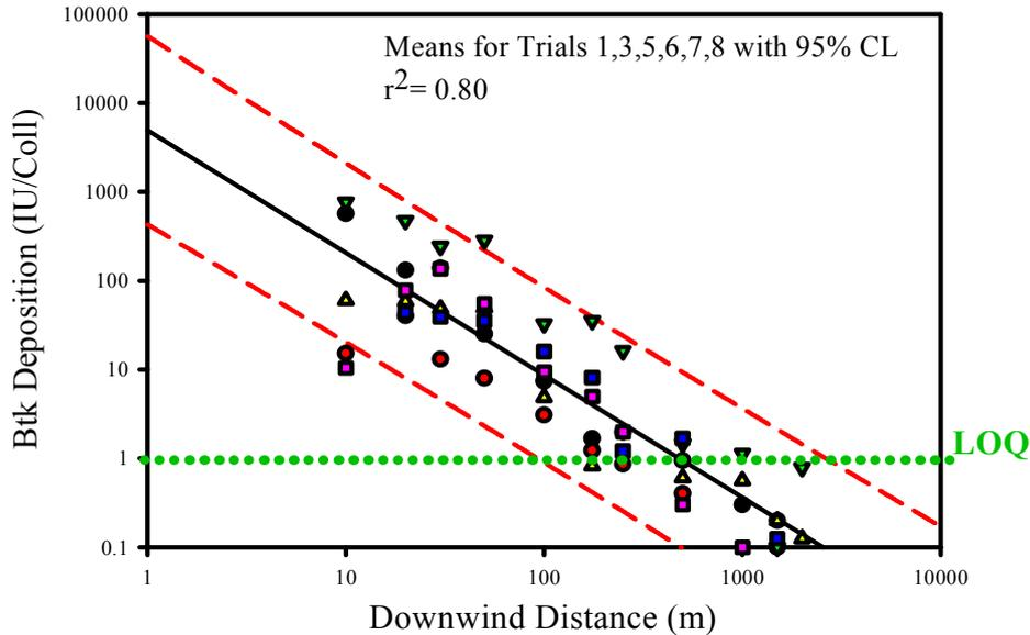
**Figure 2: Unadjusted Btk deposition on artificial foliage versus distance downwind**
