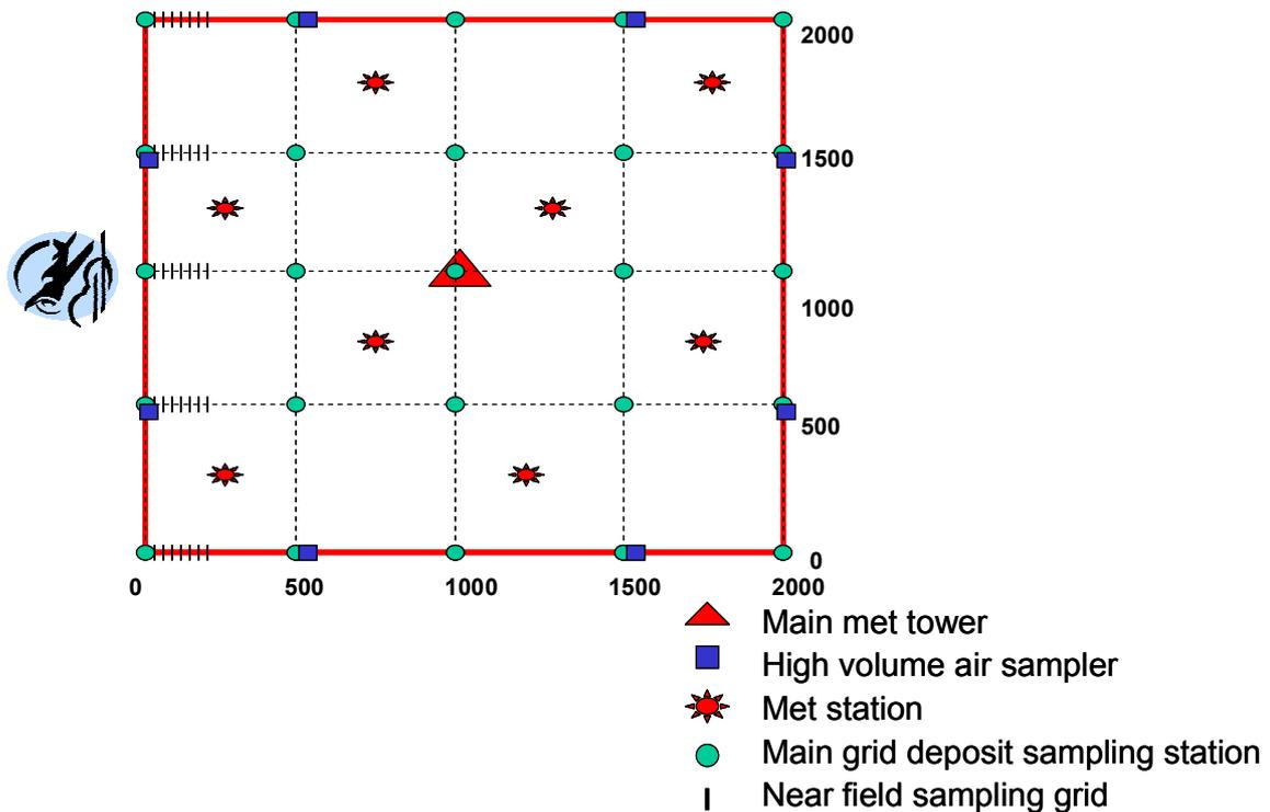
**Figure 1: Spray block layout and deposit sampling scheme**
