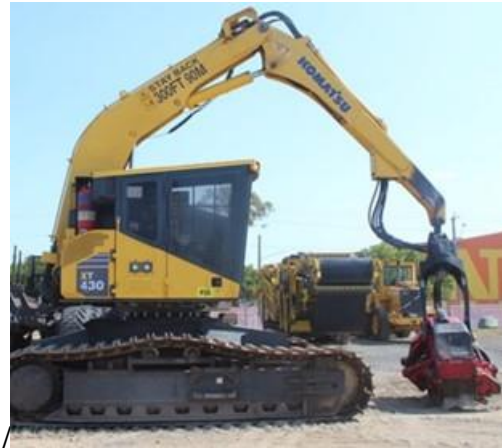
Type of harvesting machine, Valmet/Komatsu 430 Rayonier also uses a small Waratah harvesting head.
