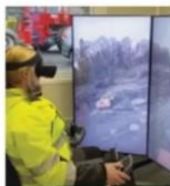
Virtual reality-based teleoperation of forwarder (Courtesy of Skogforsk's Telematikk Forestry Teleoperation Lab)
