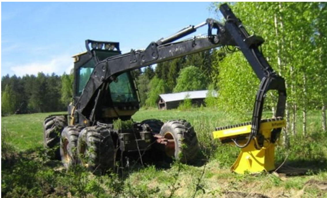
Figure 20 M Planter on a harvester
