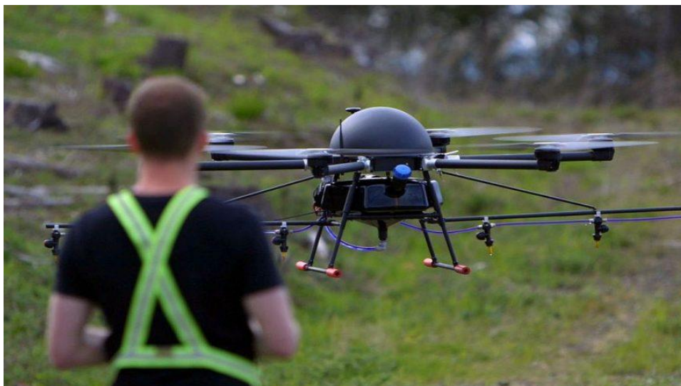
Figure 40 Droneseed UAV can hold 1000 seeds
