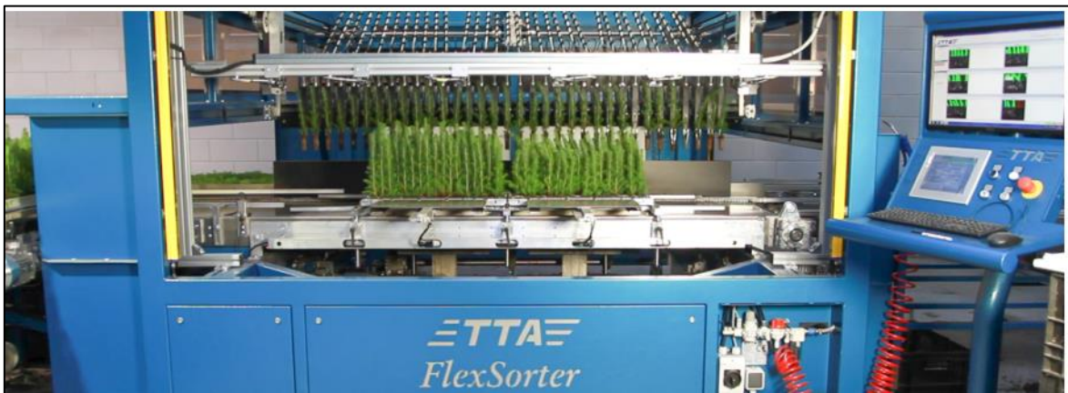
Figure 27. FlexSorter with 3,000 – 12,000 plug capacity. Retrieved from https://www.tta.eu/equipment/projects/packing-line-for-trees
