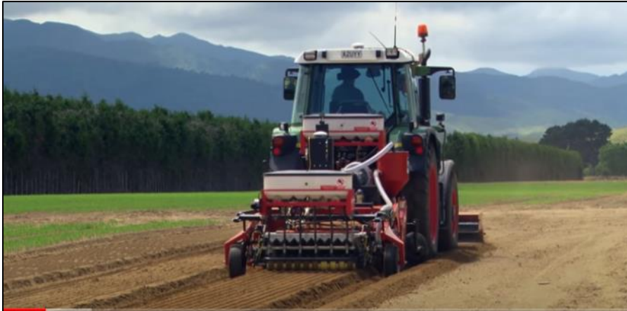
Figure 13. GPS guided tractor with bed preparation (back) and seed planting (front) modules. All modules are mounted on lateral actuators that precisely maintain the position of the modules relative to the seed bed being formed. Retrieved from https://www.murraysnurseries.co.nz/ on 05-04-22
