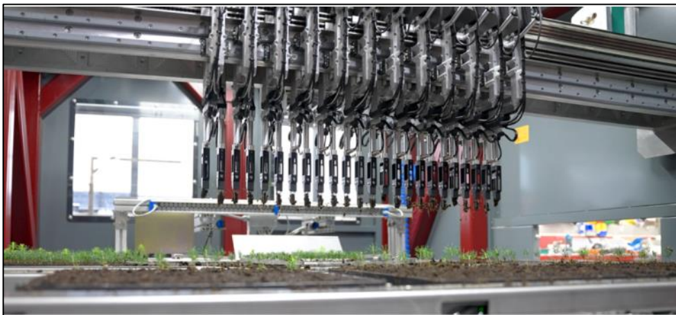
Figure 22. Multiline gripper fingers of transplanting and sorting machine. Retrieved from https://bccfibercell.com/transplanting-2/ on 110422
