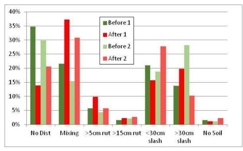
Figure 15: Soil disturbance recorded over the two transects before and after skidding
