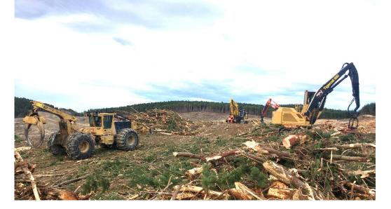
Figure 4: Landing used during the initial study at Castle Downs Forest. The skidder was lined up with the TimberMax winch assist unit (centre). The stems were dropped to the left of the processer (shown on the right).
