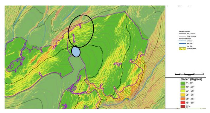
Figure 2: Section of harvest area showing slope by category. The blue circle shows location of the landing, the area circled was the skidder study.
