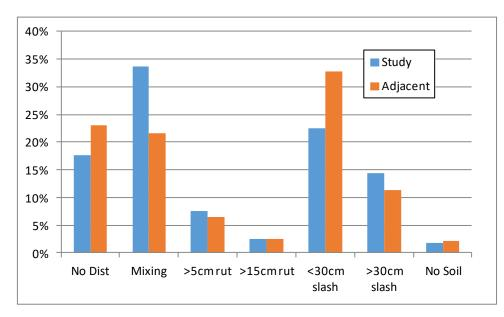
Figure 20: Overall soil disturbance on the study site (after skidding) and on the adjacent area where harvesting had been completed
