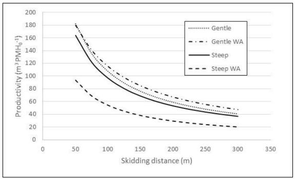
Figure 9: Delay-free productivity as a function of distance, slope gradient and winch-assistance
