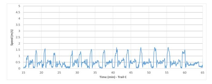
Figure 13: Skidder speed chart for Blackmount (Path 3) where the skidder was winch-assisted by the TimberMax on the steeper slope.
