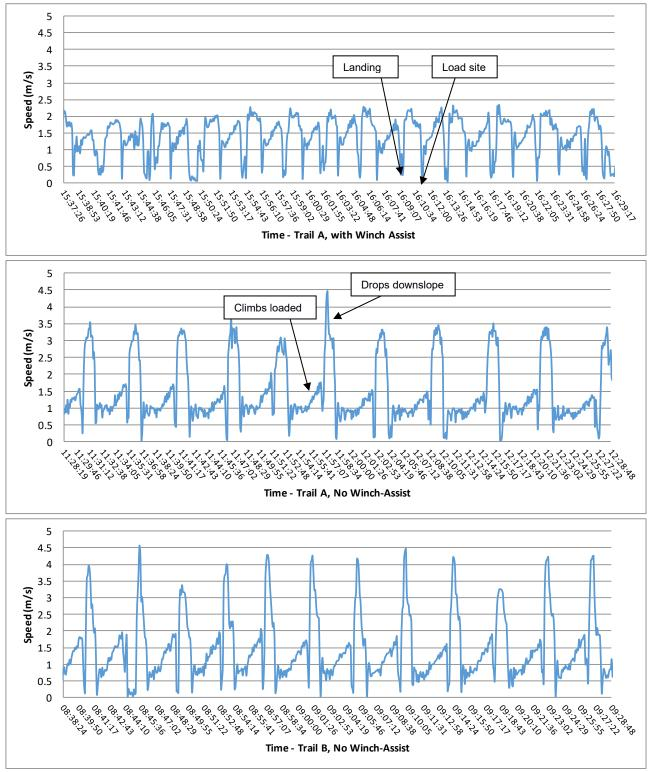
The speed graphs offered a detailed insight into skidder movements (Figure 12).
