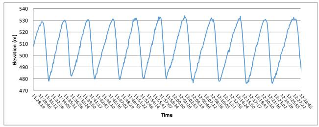
Figure 11: Skidder elevation changes of from one period on Day 1. Each sinus curve is one extraction cycle: the skidder descends to pick up the load (dip), then comes back up to take its load to the landing (peak).
