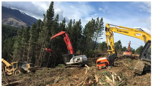
Figure 7: System set-up in Blackmount Forest, with the TimberMax winch-assist on the edge of the landing, and the shovel loader moving downslope to pre-bunch along the main path for the Tigercat 632E skidder.
