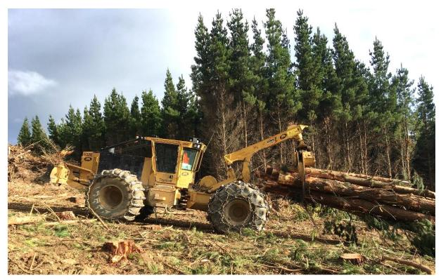
Figure 1: Tigercat 632E skidder hauling logs to landing.
