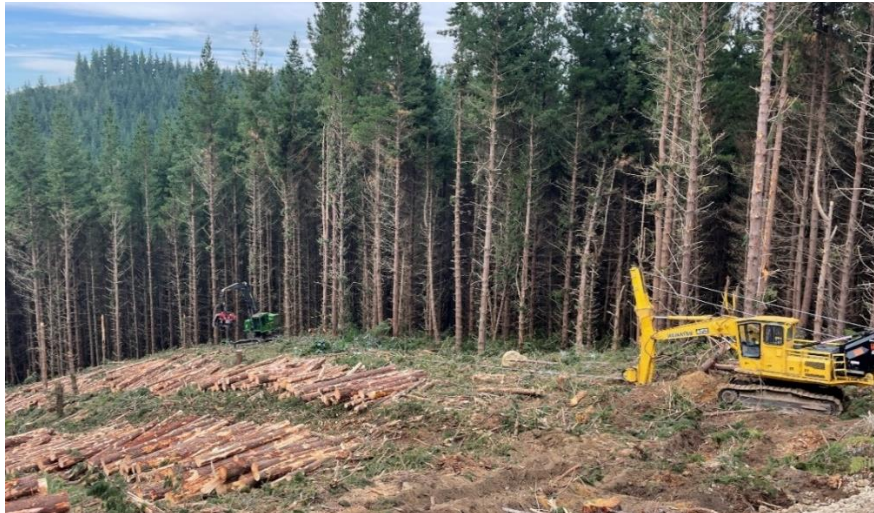
Figure 2: EMS Tractionline supporting the felling-processing machine (cut-to-length). The felled trees are cut-to-length and laid across the slope.
