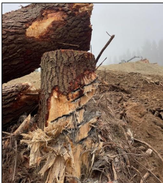
Figure 16: Wear on a stump used to redirect the wire rope.
