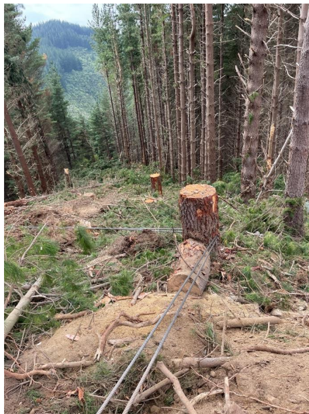
Figure 5: High stump being used to redirect the EMS Traction Line winch assist rope.
