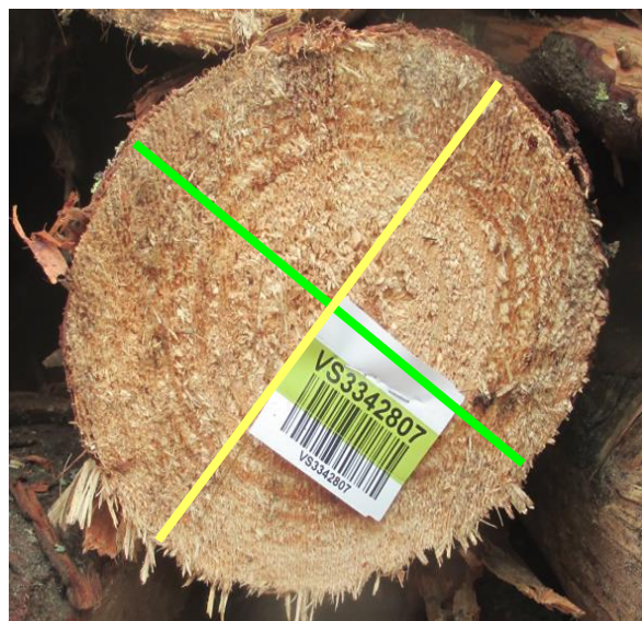
Figure 1. Under bark measurement of log diameters for JAS scaling of volume on a log with no nodal swelling.
