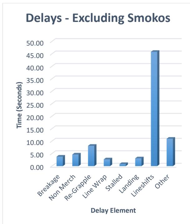
**Figure 14: Delays per cycle.**
