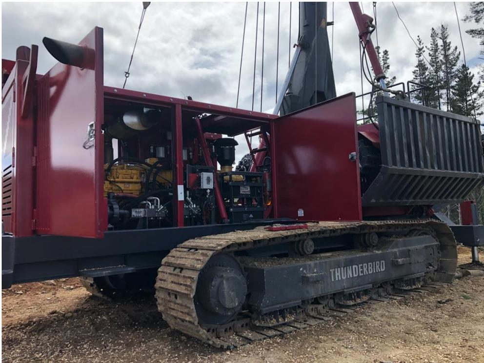
*Figure 10: The refurbished Thunderbird TTY70 has worked well in early trials.*
