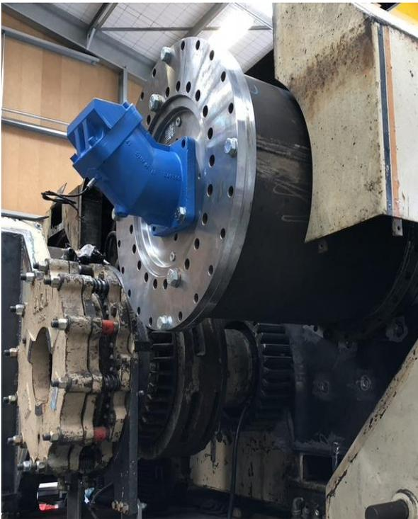
**Figure 5: Planetary drive on the skyline**
