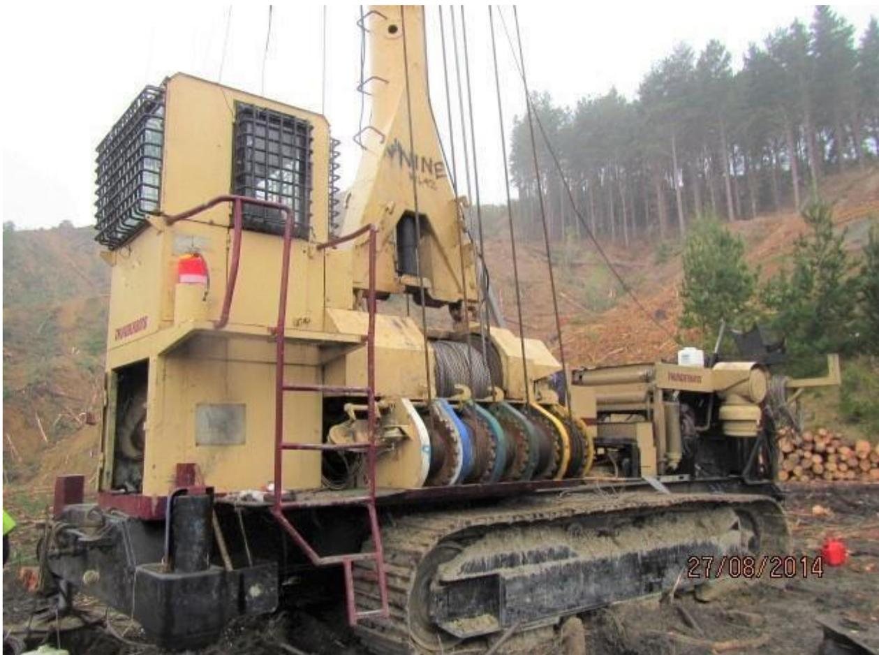
**Figure 1: The Thunderbird 70' tower machine was one of the most popular model haulers in New Zealand cable harvesting operations in a 2012 survey.**
