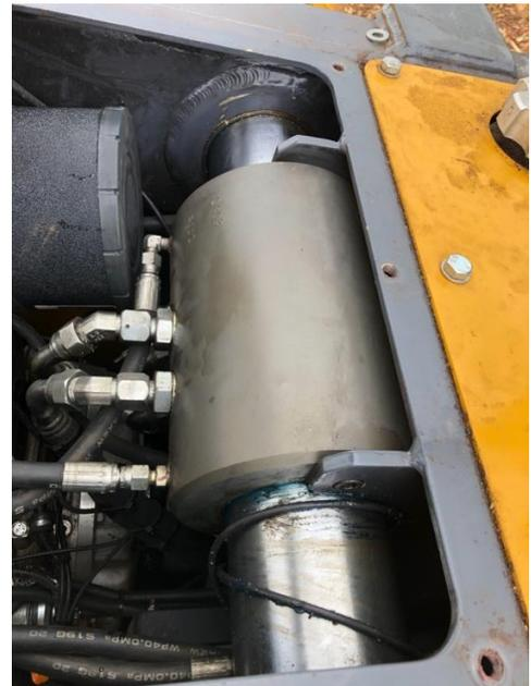
**Figure 8: The rotary oil fittings on the hanger bracket shaft.**
