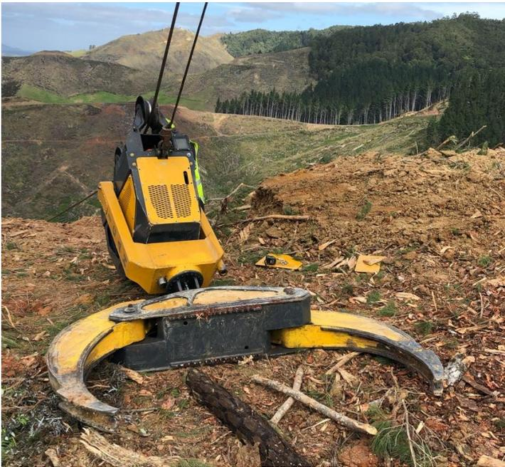
**Figure 11: The grapple carriage had a few issues and required modification.**
