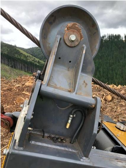
With little separation between the skyline and where the main rope attaches to the carriage, line wrap is a common problem with grapple carriages, particularly over longer haul distances. Line wrap causes significant wear to the ropes and can cause premature failure if it goes undetected.
