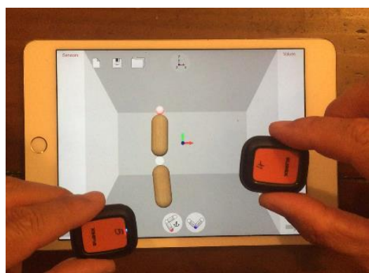
Figure 5: KineXYZ display of two IMUs.
