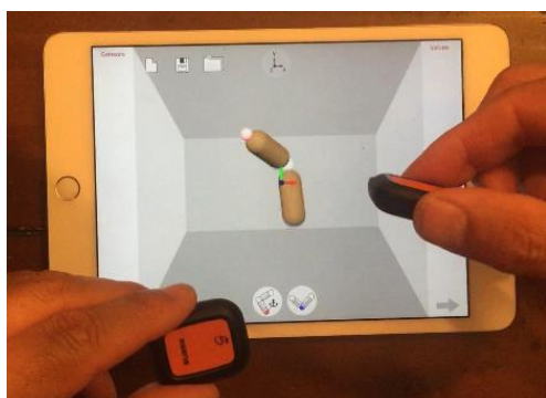
Figure 6: Right IMU (upper segment) rotated and the left IMU (lower segment) held motionless.
