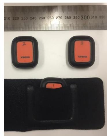
Figure 3: Xsens IMUs and strap to hold IMU on an arm, leg or machinery part
