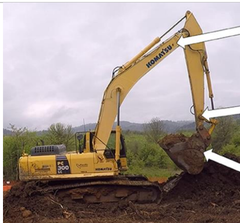
Figure 8: IMU locations to record the moment of boom and stick of an excavator (Rashid & Louis, 2020).
