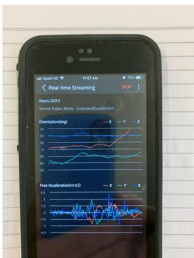
Figure 4: Line plot from individual IMU. Three lines correspond to movement in the X, Y & Z axes. Top plot is orientation and bottom plot is acceleration.
