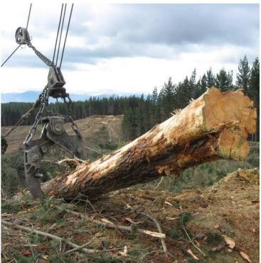
Figure 1: A typical rope-controlled grapple
