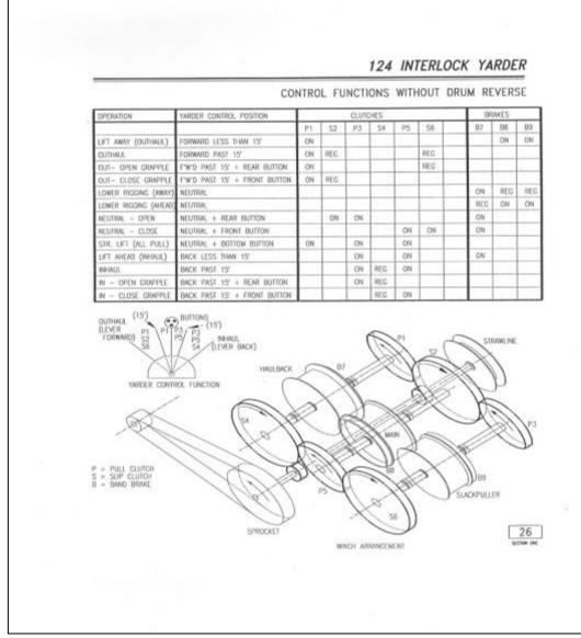
Figure 4. Madill 124 Swing-Yarder drum and brake configuration (Source: Madill Equipment)
