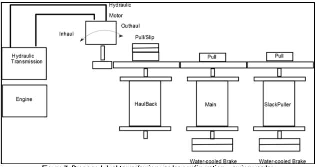
Figure 7. Proposed dual tower/swing yarder configuration – swing yarder
