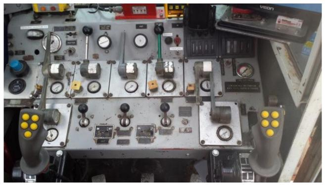
Figure 3. Old tower-hauler controls and new joystick-type controls fitted toa Madill 171 machine converted by Brightwater Engineering (Source: Bill Winmill).
