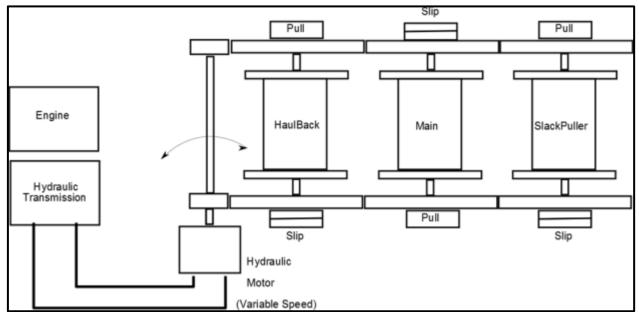
Figure 5. Proposed Swing Yarder design with additional hydraulic motor and transmission
