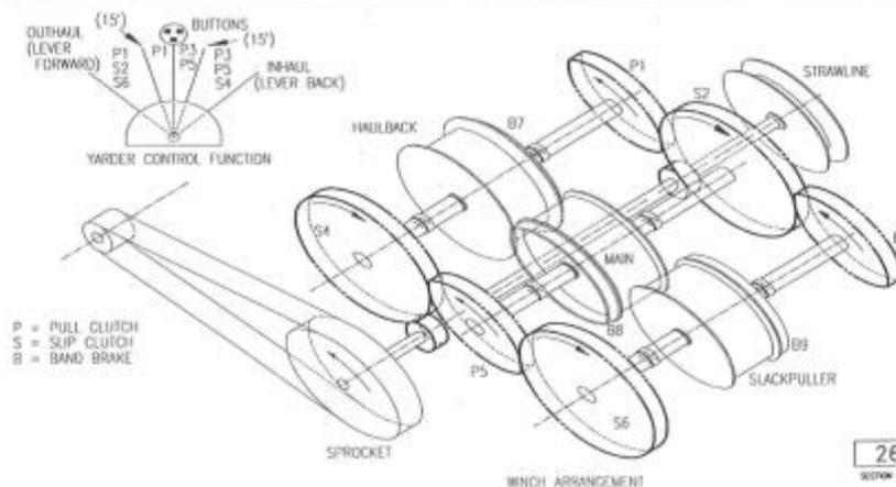
**Figure 4. Madill 124 Swing-Yarder drum and brake configuration (Source: Madill Equipment)**
