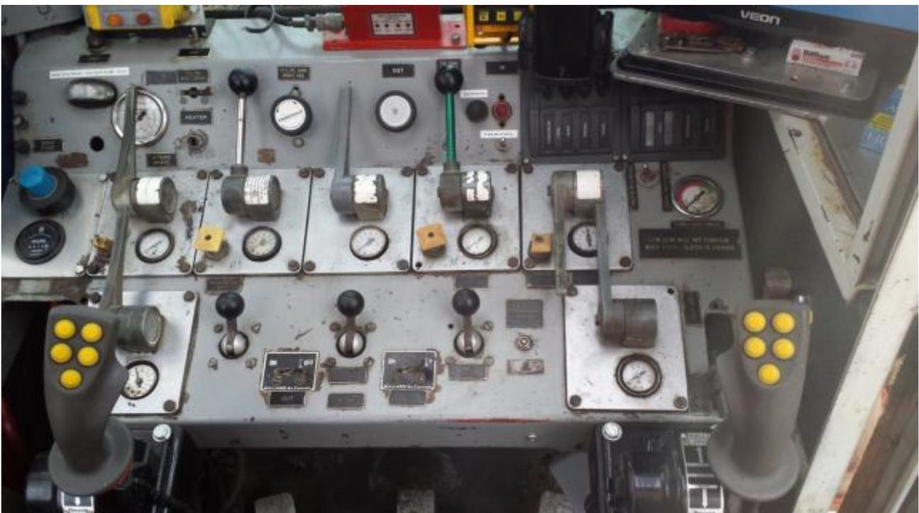
**Figure 3. Old tower-hauler controls and new joystick-type controls fitted to a Madill 171 machine converted by Brightwater Engineering (Source: Bill Winmill).**
