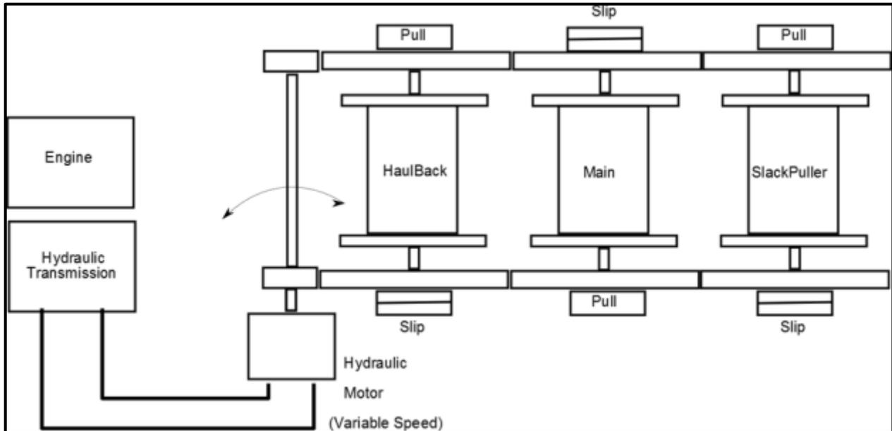
Figure 5. Proposed Swing Yarder design with additional hydraulic motor and transmission
