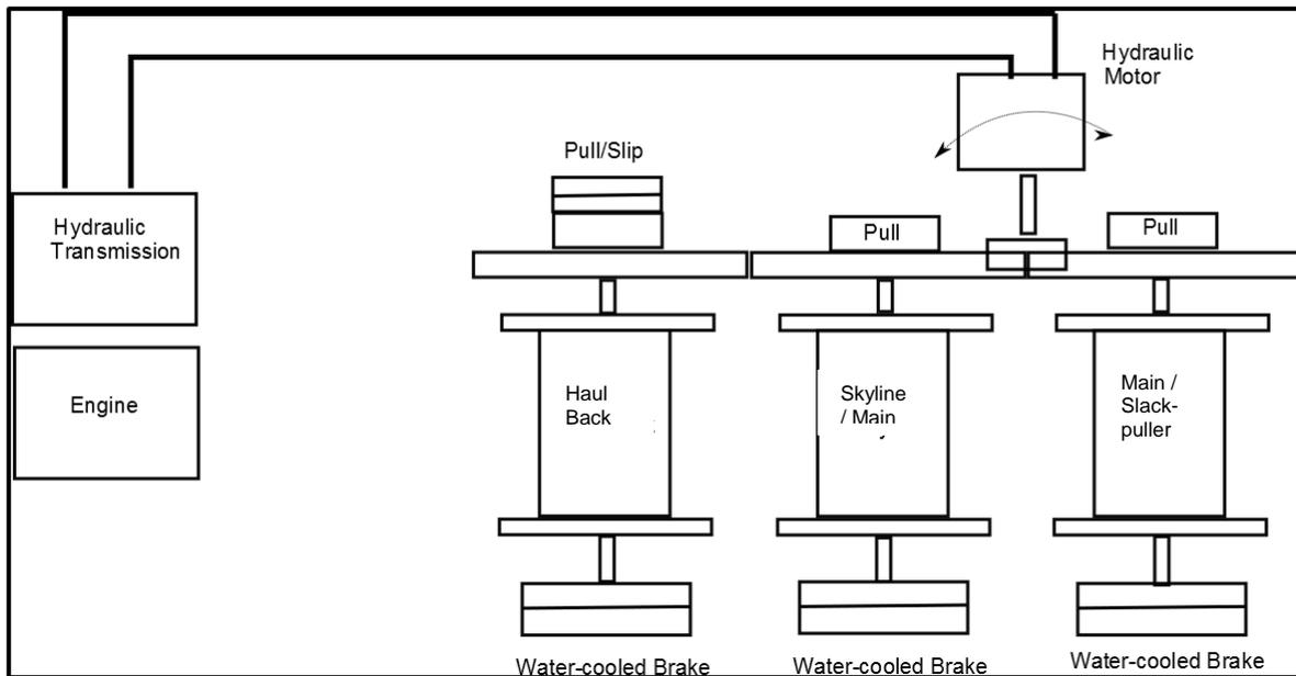
Figure 6. Proposed dual tower/swing yarder configuration – tower
