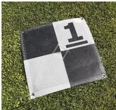
Figure 1: Ground Control Point target with approximate dimensions of 0.75 x 0.75 m.
