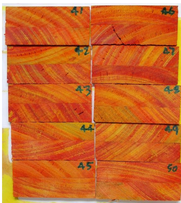
Figure 20: Penetration \sap spot test images of laminated Eucalyptus nitens in cross section
