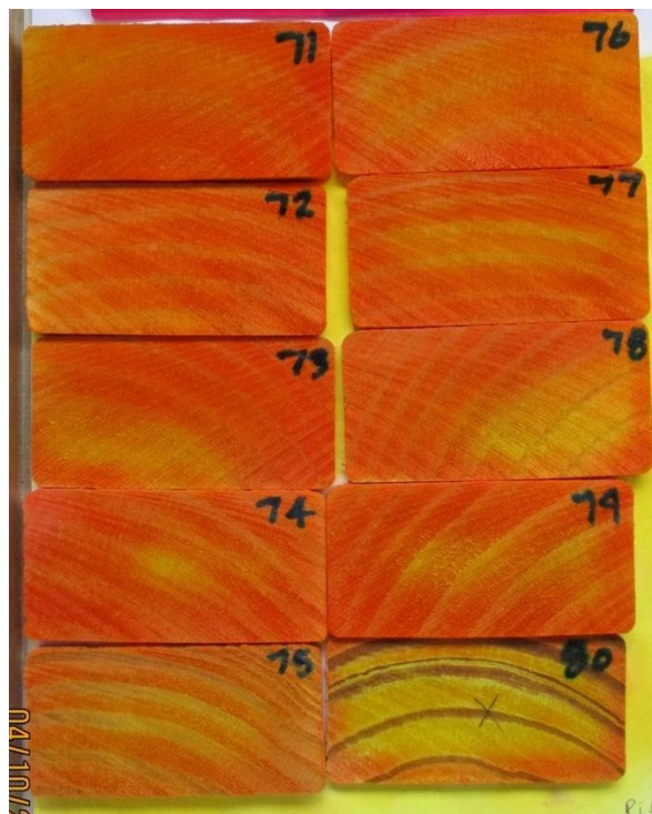
Figure 22: Penetration \sap spot test images of radiata pine in cross-section
