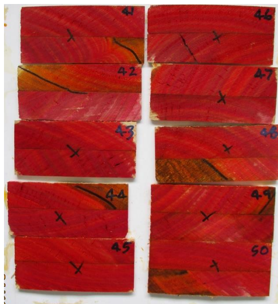
Figure 19: Heart\sap spot test images of laminated Eucalyptus nitens in cross section
