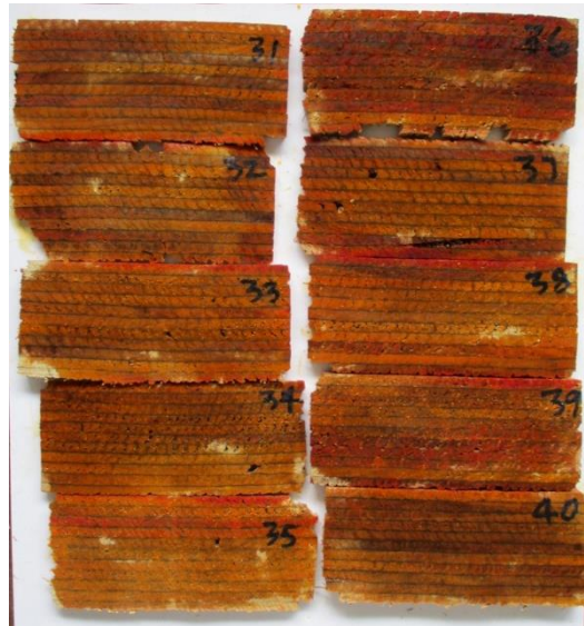
Figure 17: Heart\sap spot test images of Eucalyptus fastigata LVL in cross section
