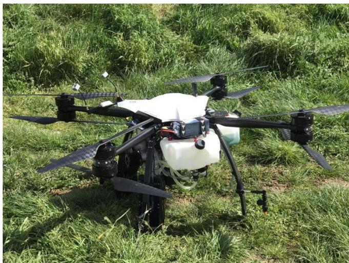
**Figure 6.** SPS Automation's custom Aeronavics Icon spray craft set up for work at the trial. The location nozzles can be seen attached to the legs, approximately under the propellers.
