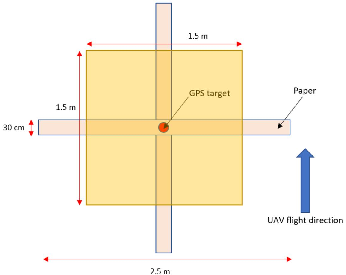
Figure 1: Layout for simple checking of spray patterns. Two strips of paper are arranged in a cross pattern over a GPS (GNSS) target. The UAV then overflies and deposits 45 mL of dye mixture (the idealised deposition shown as a yellow square) that can be visualised and measured.
