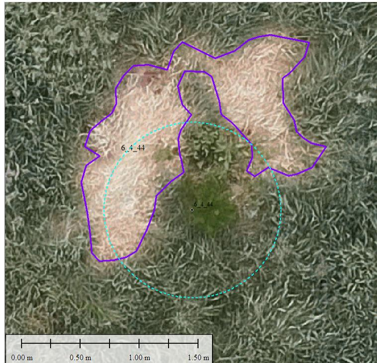
**Figure 16.** Example of spot annotation (purple polygon) showing the seedling crown is left out of the annotation, whereas the prescribed area (blue dashed circle) takes into account the seedling crown.
