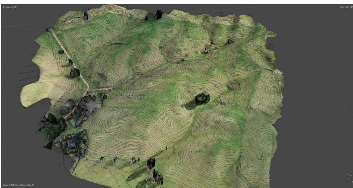
Figure 13: Generated 3d mesh, overlaid with 1m contour lines.
