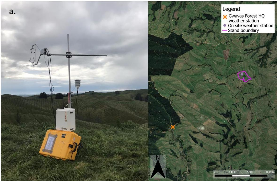
**Figure 8.** Weather station set up on the study site (a) and location of the Gwavas Forest HQ weather station in relation to the study site (b).
