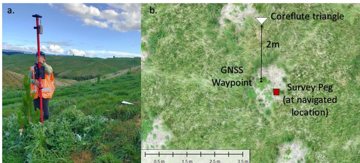
**Figure 4.** (a) Using mobile mapping system to navigate to the detected seedling waypoint in the field, with coreflute plastic marker in the right-hand side of the image; (b) diagram of the experimental layout, with the GNSS waypoint of the detected tree derived from the aerial imagery (black spot), the coreflute marker (white triangle; to aid in locating seedlings in aerial imagery) and the survey peg of where the mobile GIS navigated to (red square).
