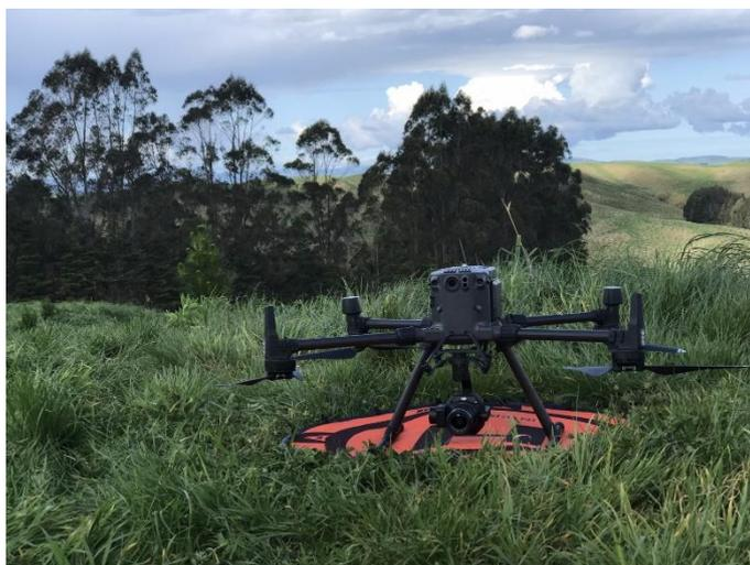
**Figure 5.** DJI Matrice 300 UAV with mounted DJI P1 camera ready to take-off for mapping the site prior to spraying
