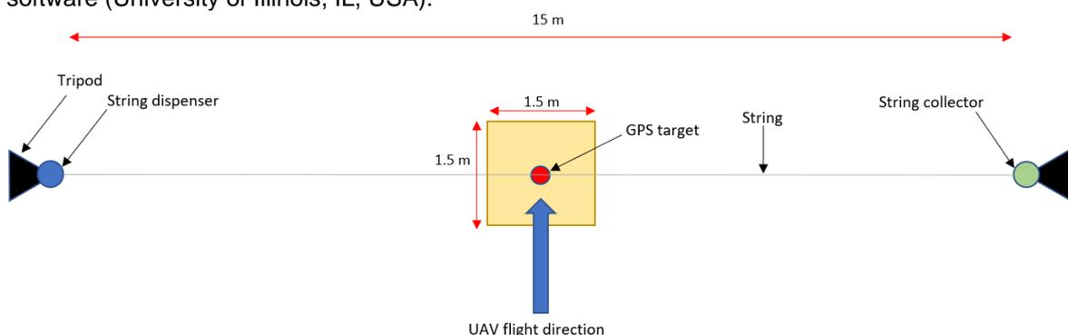
Figure 2: Layout for spray patterning with the string system. Mounted to tripods equidistant from the GPS (GNSS) target, the string dispenser (always mounted on the left) and the string collector (always mounted on the right), will be positioned such that a 15 m length of string passes over the target. Equipment will be set up so the UAV flies into the predominant wind direction.
