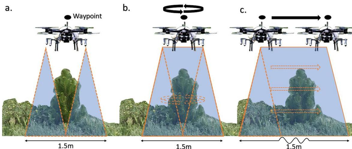
**Figure 7.** Spray deposit methods that can be used for spot application from a UAV: (a) stop and spray; (b) stop and rotate; (c) intermittent swath spray with waypoints before and after the target tree to turn on and off the flow. Note: spray deposits are for demonstration purposes and diagrams not to scale.
