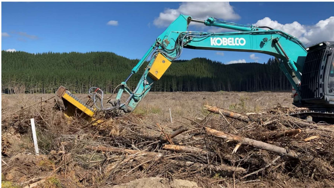
Figure 9: The mechanical planter moving piles of slash.
