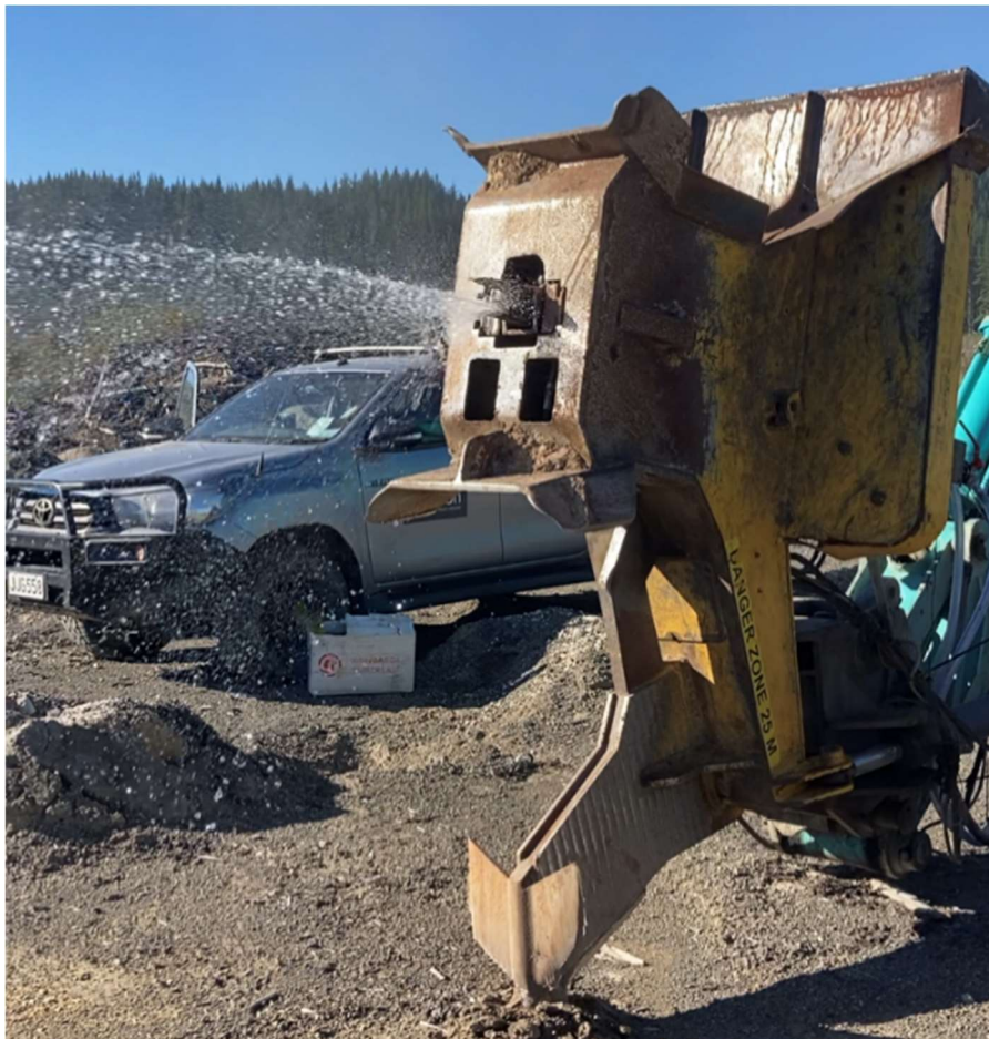
Figure 4: The jet of liquid indicates the testing of the suitability of the hydrogel's viscosity for the trial.
