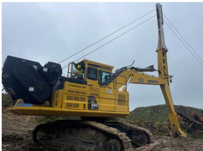
Fig 4. Harvestline mounted on Komatsu PC400LC.
