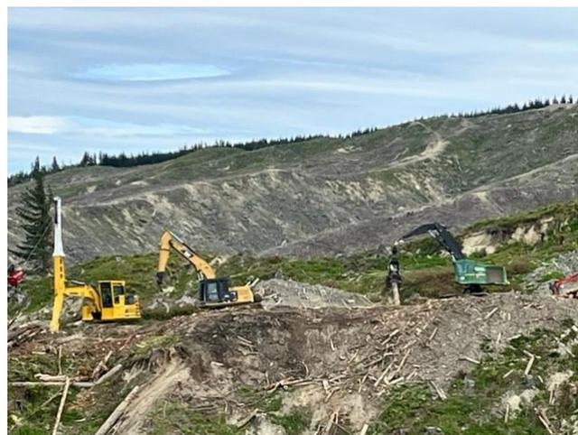
Fig 2. Harvestline set-up and supporting equipment.
