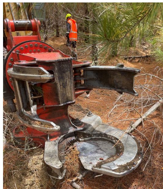
Fig 1: Ensign fixed shearing head
