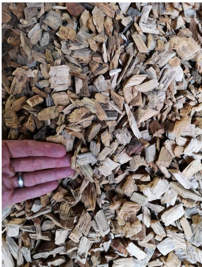
**Figure 2: Standard size specification boiler fuel**
