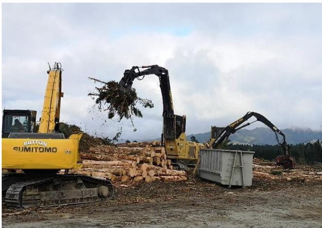
**Figure 5: Example of harvesting residues loaded to bin**
