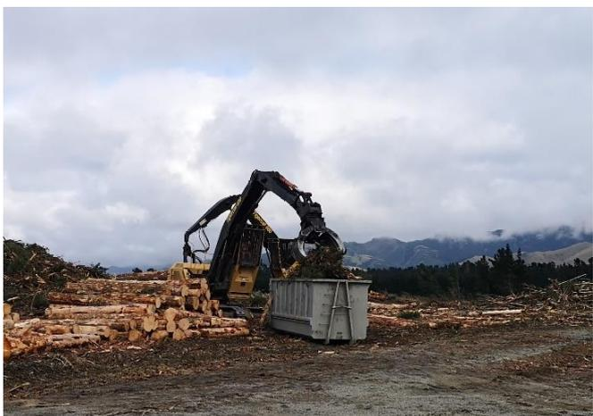
**Figure 6: Compaction of the residues in the bin**
