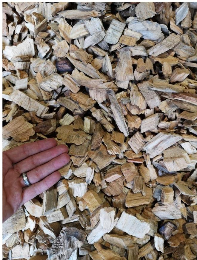
**Figure 3: Larger size specification boiler fuel**
