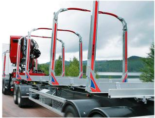
Figure 3: ExTe automatic log load restraint system. Source: www.exte.se
