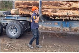
Figure 7: Step 2 of the side-arm technique: Coiling/reeling of the chain to concentrate its mass and throw it all over.
