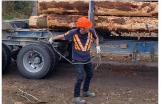
Figure 8: Step 3 of the side-arm technique: The "loading" of the throwers arm, the start point in the throw where the throwers arm and shoulder are both at full extension.
