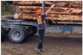
Figure 9: Step 4 of the side-arm technique: the final point in the throw of the chain, the release of the mass.
