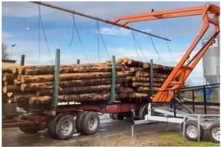
Figure 2: Timberlands' chain placement system uses a trailer mounted hydraulic lifting arm to deliver chains to the other side of two log packets with minimal effort.
