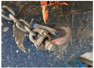
Figure 10: Misalignment of the D-shackle on the trailer eye prior to tensioning can cause the shackle to slip/spin under load, rapidly slackening the chain and destabilising the driver tensioning the assembly.
