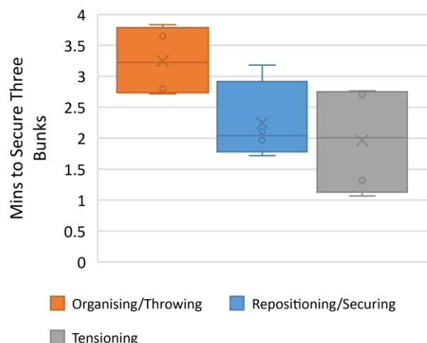
Figure 5: Elemental time study of securing 3 log bunks (4 trucks observed).
