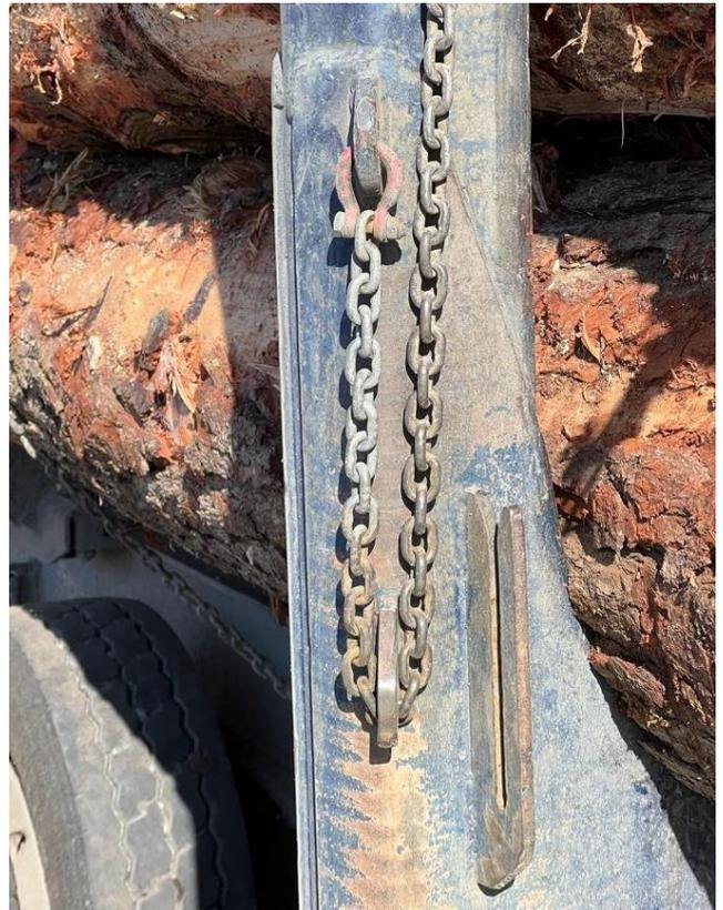
**Figure 11: Fixed chain attachment point with redirector to potentially eliminate shock loads from shackle misalignment.**
