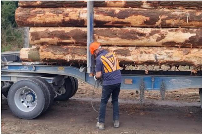
**Figure 6: Step 1 of the side-arm technique: removal of the chain from its storage position and the subsequent attachment of it.**
