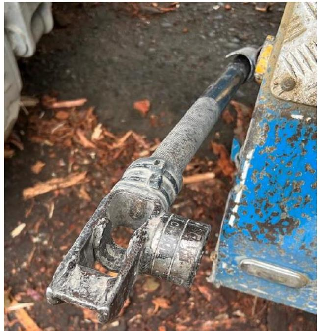
**Figure 12: Multi-use power bar, used for increasing leverage over the twitch bar and now designed to hold securely onto the twitch to reduce incidences of slipping while levering the unit closed.**
