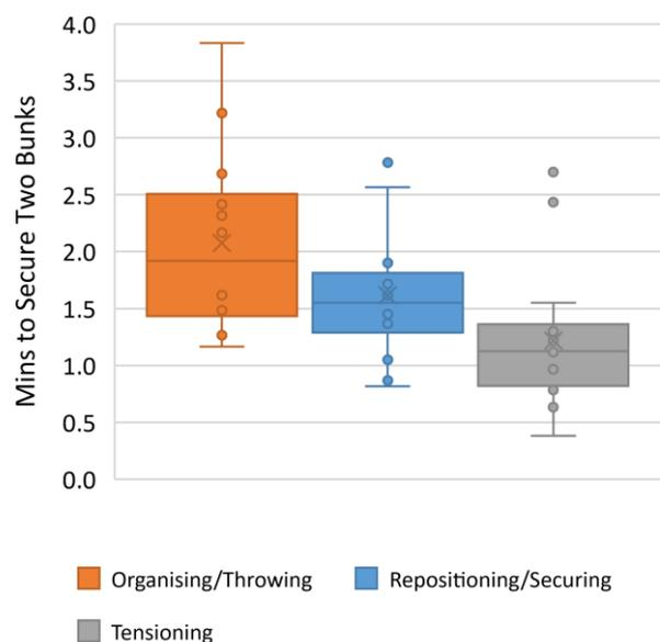
Figure 4: Elemental time study of securing 2 log bunks (14 trucks observed).
