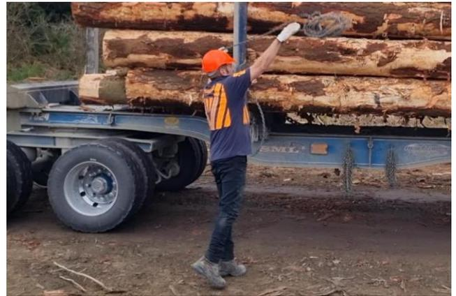
**Figure 9: Step 4 of the side-arm technique: the final point in the throw of the chain, the release of the mass.**
