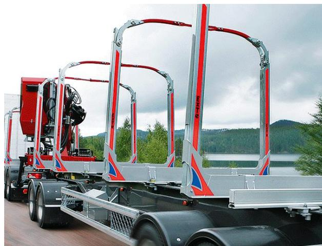
**Figure 3: ExTe automatic log load restraint system. Source: [www.exte.se](http://www.exte.se)**
