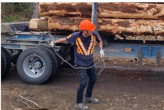
**Figure 8: Step 3 of the side-arm technique: The "loading" of the throwers arm, the start point in the throw where the throwers arm and shoulder are both at full extension.**
