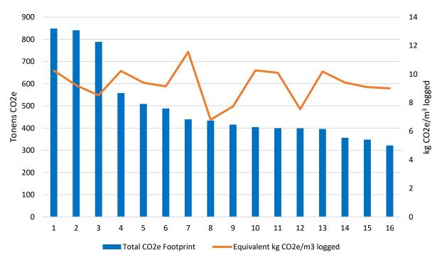
Figure 6: Cable yarder harvesting carbon emissions NZ - Fuel data from Oyier (2015)
