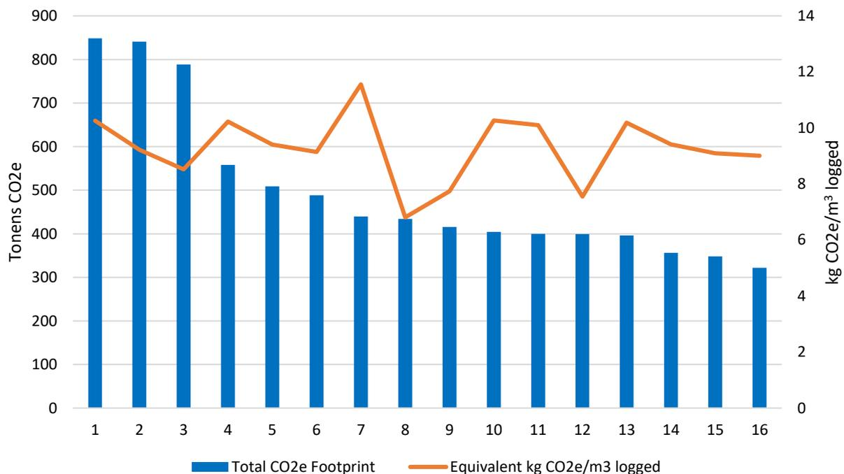
**Figure 6: Cable yarder harvesting carbon emissions NZ - Fuel data from Oyier (2015)**
