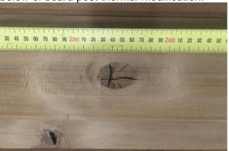
Overall the thermal modification process did not produce excessive degrade in *C. lusitanica* and *C. x ovensii*. It was known that tight knots are prone to star checking following thermal modification, but the proportion of timber downgraded due to knot checking was quite small. The effect of knot checks could be further reduced by filling the knots following modification.
