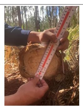
Recutting of the logs appeared to slightly increase the mean index of the cut logs, however there was no statistical difference observed. The new logs (3-6m) all had some face checking and similar amounts of logs with no cracking or splitting.
