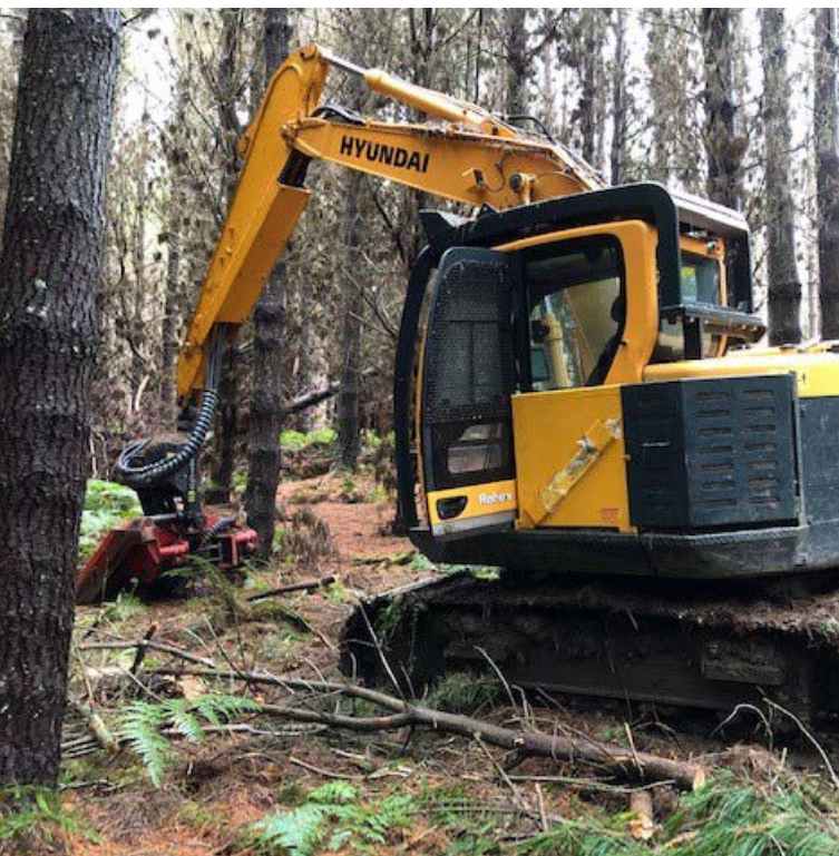
^ A small-scale harvester-processor production thinning in a Southland radiata pine forest. (Contractor: John Fodie).
