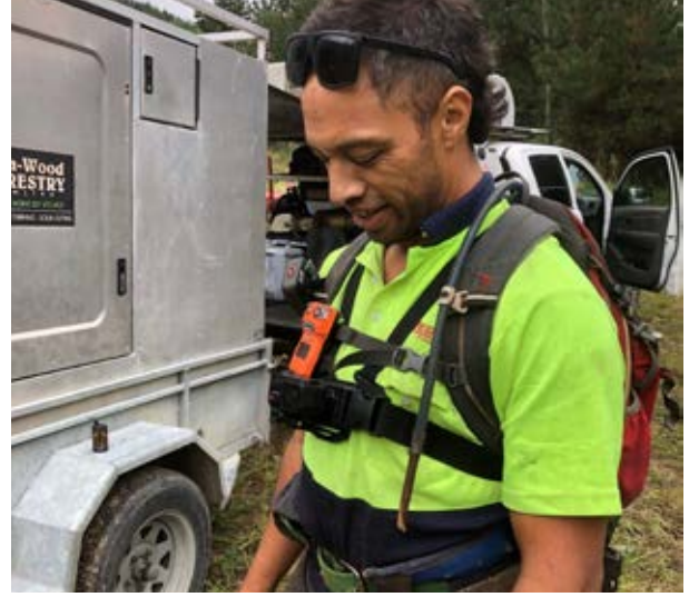
^ Chainsaw operator with camera and carbon monoxide monitor attached.
