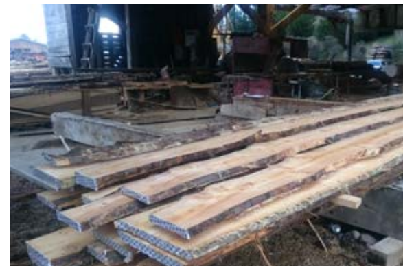
^ Cypress boards from 20-year-old trees awaiting grading and resawing, Ruapehu Sawmill.
