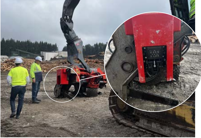
^ The Otmetka log marker prototype mounted on a Woodsman 750 head at the Kaingaroa Processing Plant (Timberlands).
