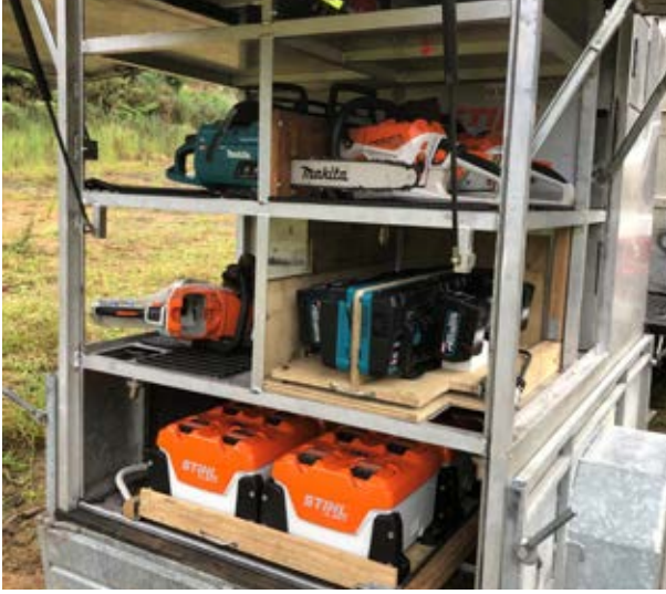
^ The specially adapted trailer, enabling 40 batteries to be charged overnight from one socket.
