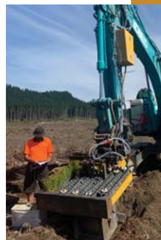
^ Preparing to plant hydrogel-treated seedlings with the M-planter.
