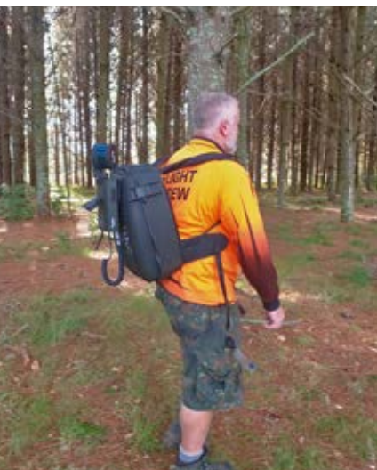
^ Scion's Pete Massam trials the backpack-mounted Hovermap laser scanner.
