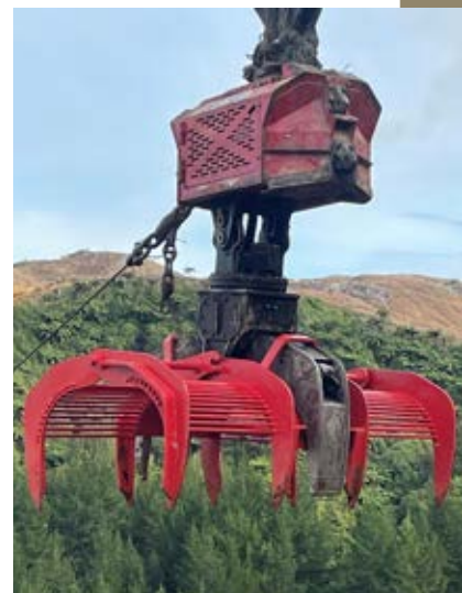
^ JDT Engineering's hauler slash grapple prototype.
