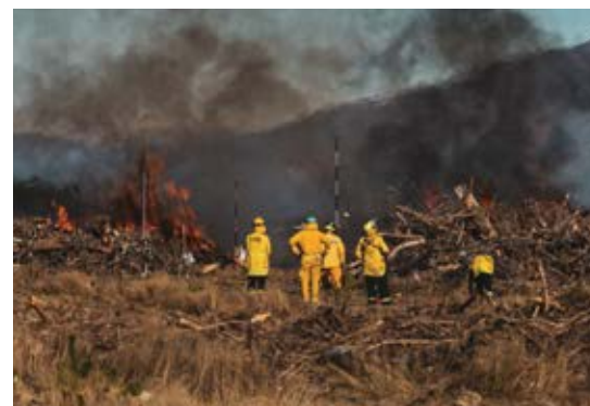
^ Scientists and fire crew monitor fire whirl development in heavily instrumented radiata pine slash fires.
