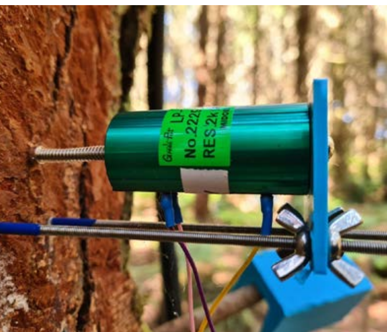
^ A dendrometer measuring precise tree stem expansion, and sometimes contraction, Kinleith Forest.
