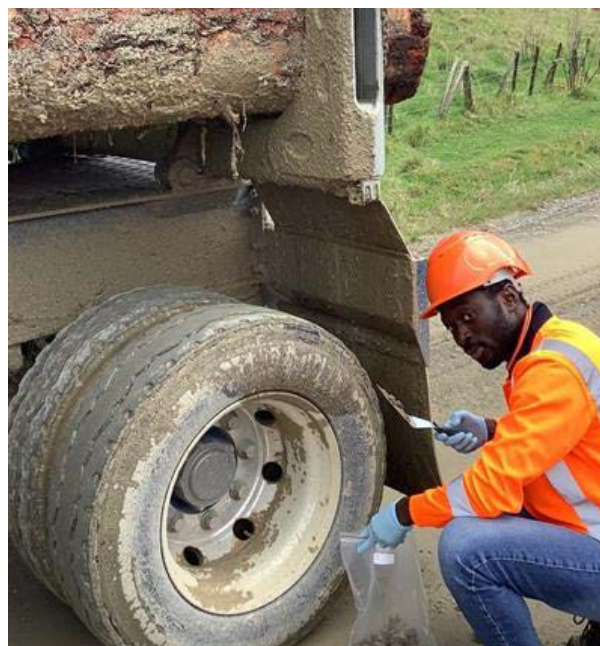
^ Dr Kwasi Adusei-Fosu takes soil samples from a logging truck in wet conditions.
