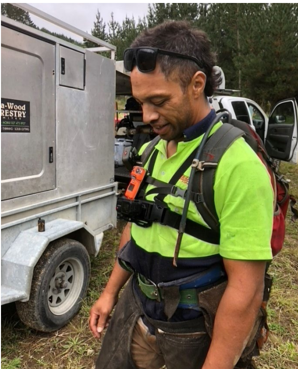
Fig 11: Intra-Wood Forestry's thinner Pae with the camera and CO monitor attached to his chest.
