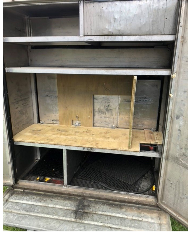
Fig 7: Plywood shelves were mounted in the front compartment of the trailer.
