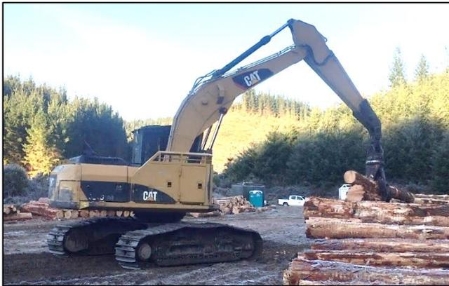
**Figure 2. Single loader skid.**
