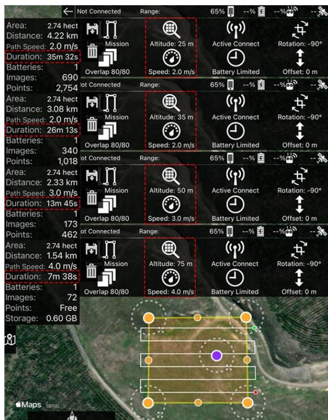
Figure 7. An example of how UAV flight duration, overall flight distance and image count (photogrammetric data captured) decreases with elevation gain over an identical 2.74 ha flight area. Note, the number of flight lines in the
