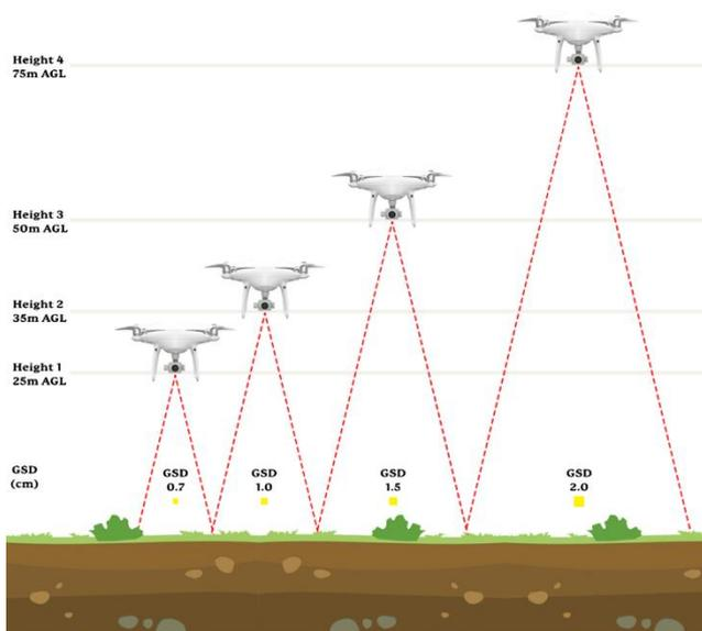
Figure 1. Diagram displaying the relationship with the increase in altitude with the increase in GSD utilising the altitudes assessed in this report.
