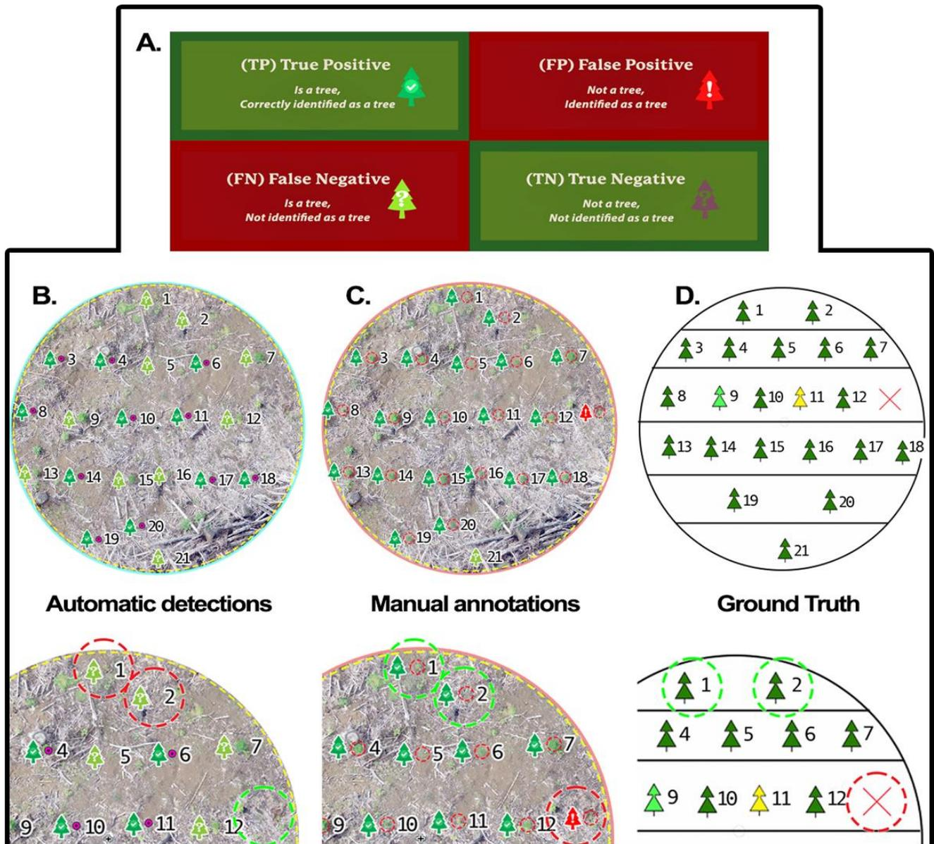
Figure 5. Graphical explanation of the accuracy assessment methodology: (a.) an example of a confusion matrix featuring detection classifications, methods for comparing automatic (b) and manual detections (c.) to field data (d). Close up images show examples of FN (b.; light green trees with red circles), TP (c.; dark green trees with green circles and FP (c.; red tree, red circle).
