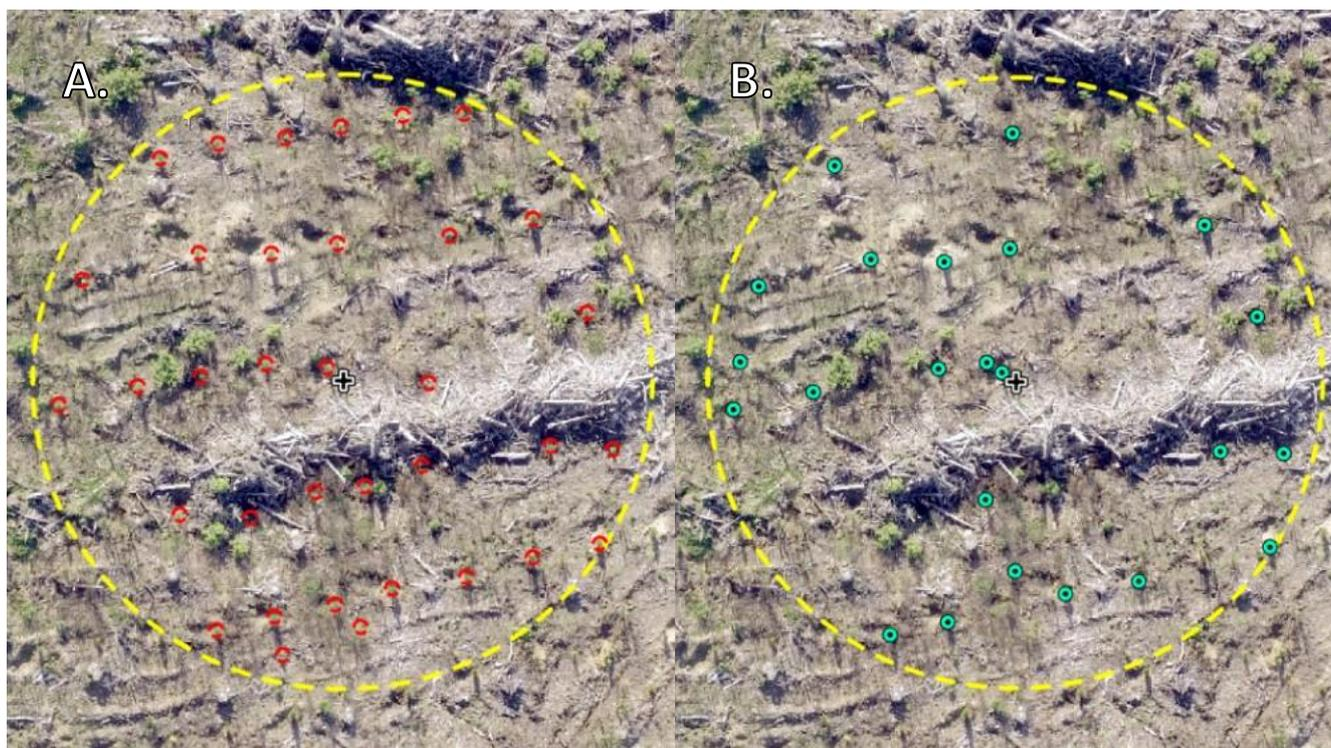
Figure 4. Example of annotations for Kinleith Forest plot 2 on a 1 cm GSD orthomosaic with a. manually annotated and b. automatically detected seedlings. Figures show plot boundaries (yellow), plot centres (black crosses), manual seedling annotations (red) and automatic seedling detections (cyan).
