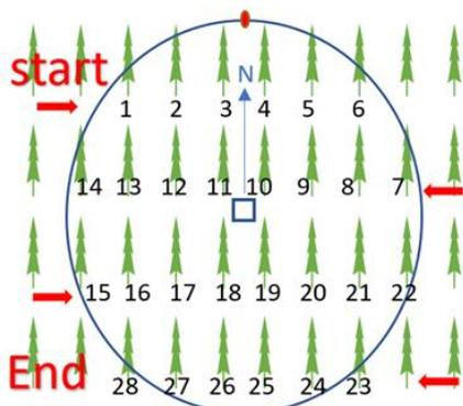
Figure 2. Plot assessment diagram for ground truth data capture, showing the start and end points for measuring plots relative to the plot centre.
