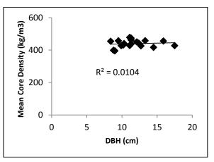
Figure 9. Wood density at 1.4 m above ground of 19 kauri stems sampled from the Mangatangi thinning trial.
