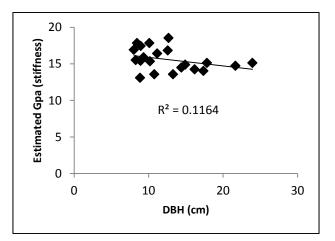
Figure 11. Stiffness of kauri stems from the Mangatangi thinning trial measured by acoustic velocity and converted to GPa.
