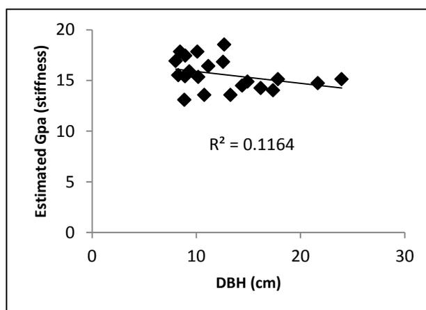
Figure 11. Stiffness of kauri stems from the Mangatangi thinning trial measured by acoustic velocity and converted to GPa.
