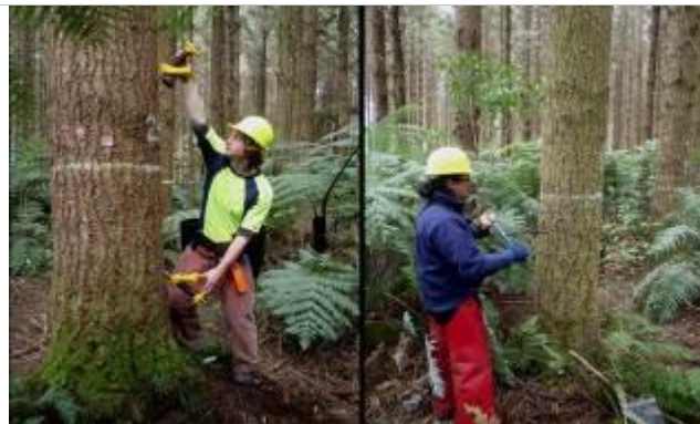
Figure 2. Assessment of acoustic velocity and core extraction to determine wood density
