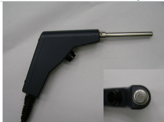
Figure 1: Fibre-optic probe used with the Bruker spectrometer, showing a close-up of the optical fibres on the probe tip (inset).
