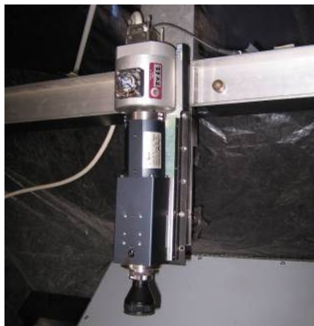
Figure 2 : NIR line camera used to acquire hyperspectral images of the heartwood blocks.
