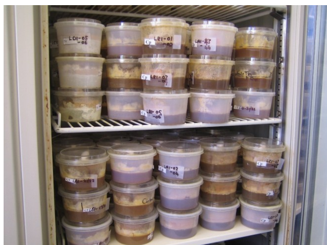
Figure 3: Decay testing of the coast redwood heartwood, and radiata pine sapwood, blocks with fungal cultures.
