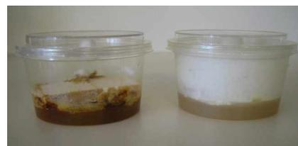
decay testing using three fungal cultures. Two brown-rot fungi were used that are supposed to attack softwoods like cypresses, and one white-rot fungus (for hardwoods) as a supposedly ineffective control. In contrast to radiata pine sapwood, none of the Leylands lost any weight as a result of the brown-rot fungi, but – surprisingly – there was a slight loss as a result of the white-rot.
