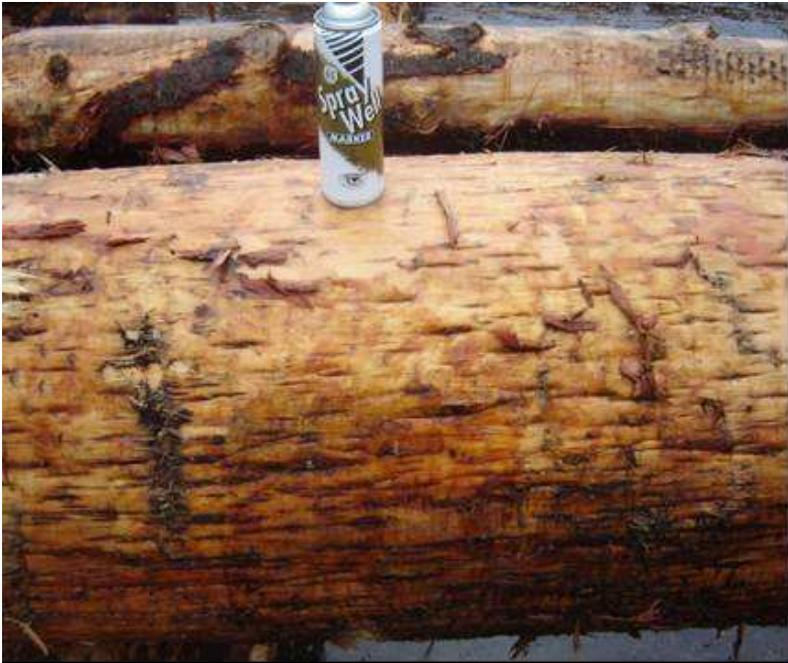
**FIGURE 9: Example showing that even small Type 2 resin pockets produced at a young age are commonly associated with pitting.**
