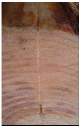
FIGURE 10: Further examples of Type 2 RP's associated with pitting.
