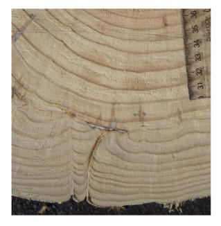
Two Type 2 RP's, showing associated occlusion scares & traces to stem circumference
