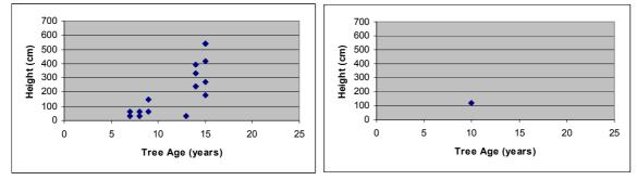
FIGURE 5: Incidence by height and formation age of Type 1 (left) and Type 2 (right) resin pockets in Canterbury logs with bark lesions. Points may represent one or more resin pockets.
