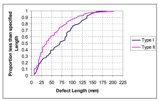
Fig. 5. Cumulative distribution of defect maximum lengths in the combined data
