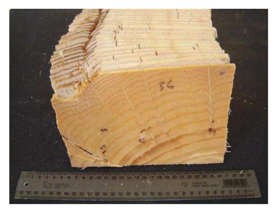
Fig. 3. Section of a log slab crosscut into slices. Several exposed resin pockets are visible on the front slice
