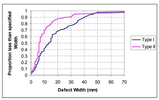
Fig. 7. Cumulative distribution of defect maximum widths in the combined data
