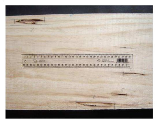
Fig. 2. Surface of a board during planning showing several mainly Type II resin pockets
