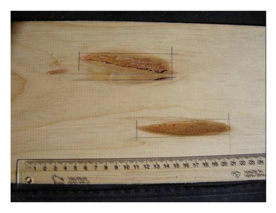
Fig. 1. Surface of a board during planing showing the process of measuring two large Type I resin pockets
