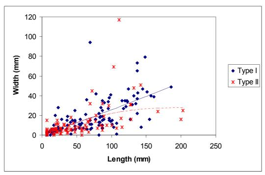
Fig. 9. Defect width versus defect length for Type I and II defects. Fitted lines using Model (1) are shown for Type I defects (solid line) and Type II defects (dashed line)
