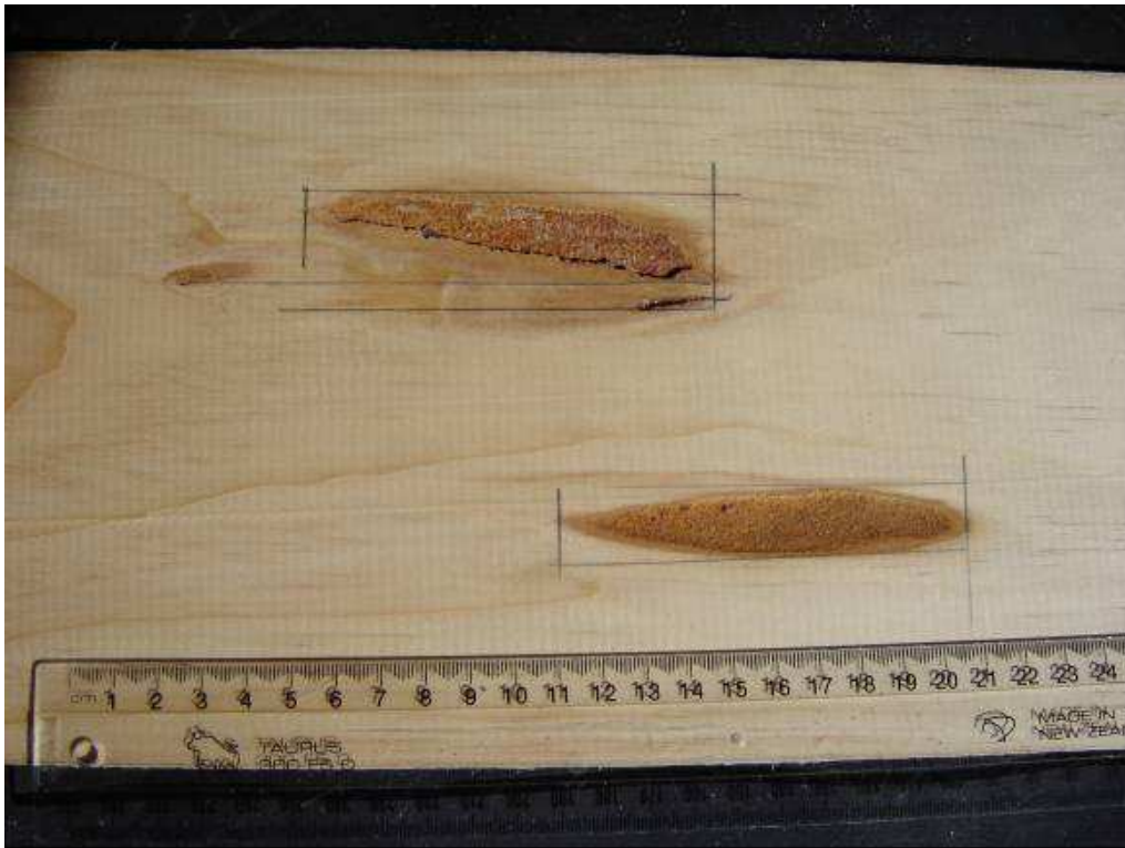
Fig. 1. Surface of a board during planing showing the process of measuring two large Type I resin pockets
