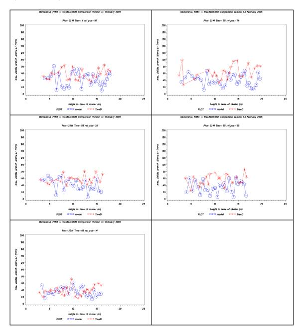
Graph showing PhotoMARVL measurements and TreeBLOSSIM predictions of branch diameter versus height of cluster for individual trees in FR54, plot 23\_14 (GF9 seedlot).
