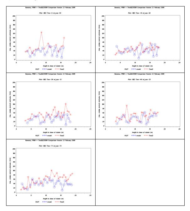
Graph showing PhotoMARVL measurements and TreeBLOSSIM predictions of branch diameter versus height of cluster for individual trees in FR84, plot 19\_21 (GF16 seedlot).
