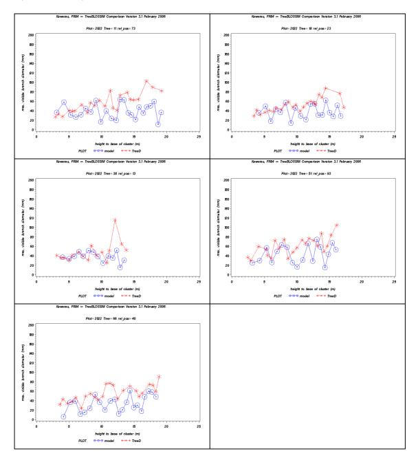
Graph showing PhotoMARVL measurements and TreeBLOSSIM predictions of branch diameter versus height of cluster for individual trees in FR84, plot 21\_24 (GF16 seedlot).
