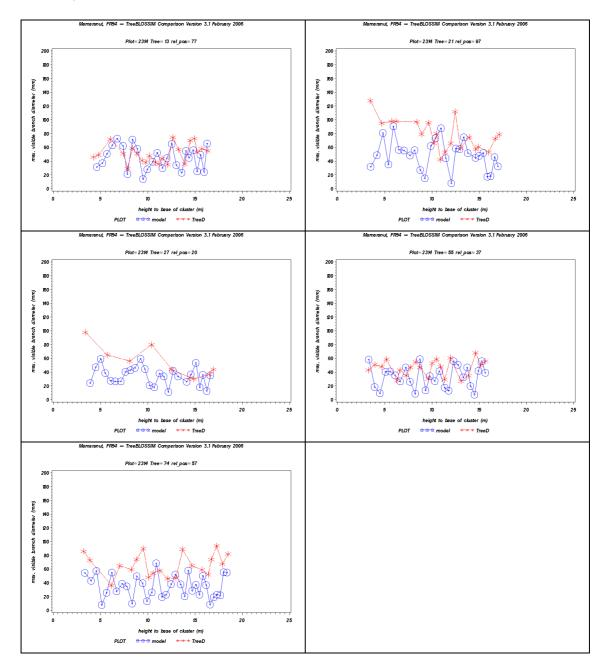
Graph showing PhotoMARVL measurements and TreeBLOSSIM predictions of branch diameter versus height of cluster for individual trees in FR54, plot 24\_14 (GF22 seedlot).
