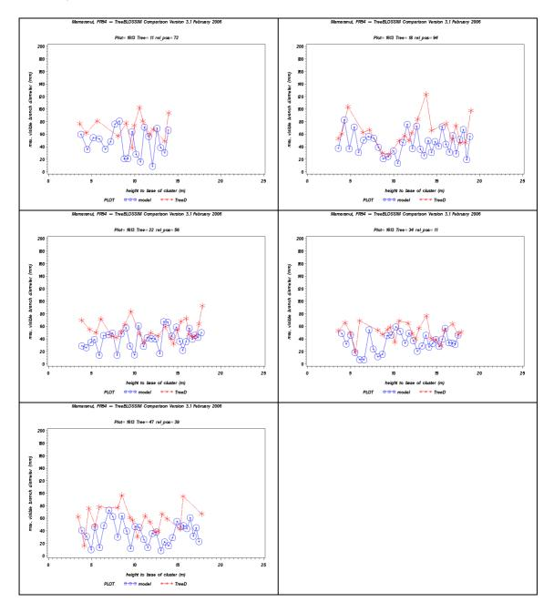
Graph showing PhotoMARVL measurements and TreeBLOSSIM predictions of branch diameter versus height of cluster for individual trees in FR54, plot 17\_13 (GF22 seedlot).
