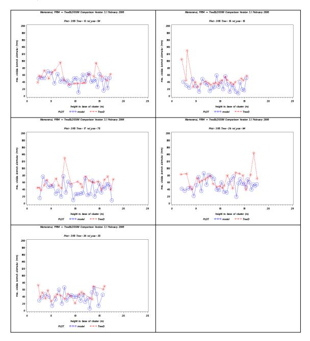
Graph showing PhotoMARVL measurements and TreeBLOSSIM predictions of branch diameter versus height of cluster for individual trees in FR54, plot 41\_17 (GF17, cuttings seedlot).
